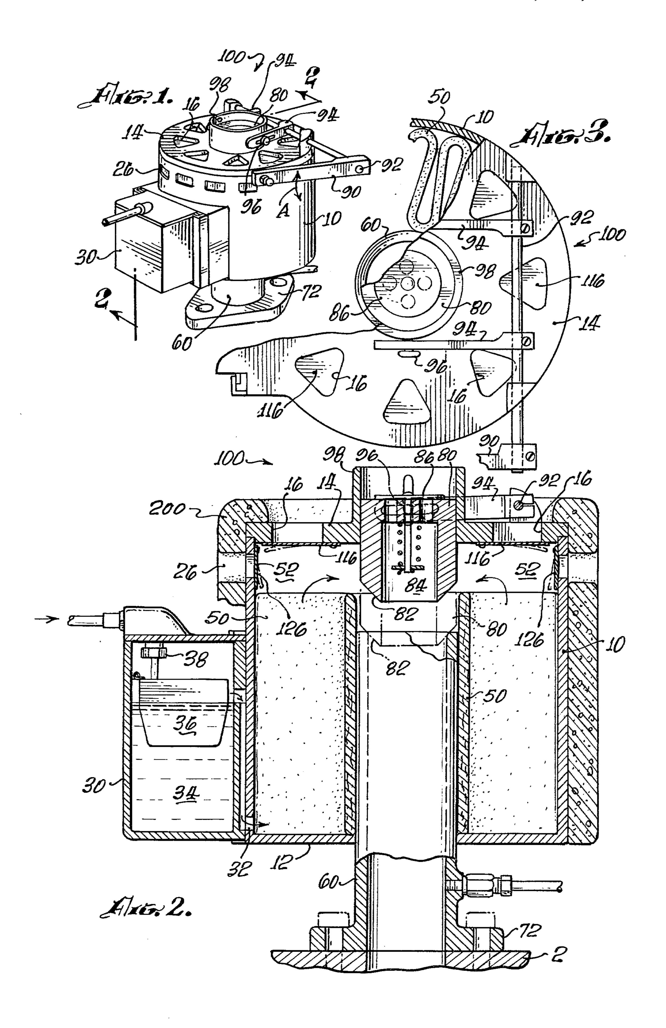
spark-ignition engines. Fuel is admitted into the evaporation chamber at the bottom via a conventional float valve and metering bowl.
