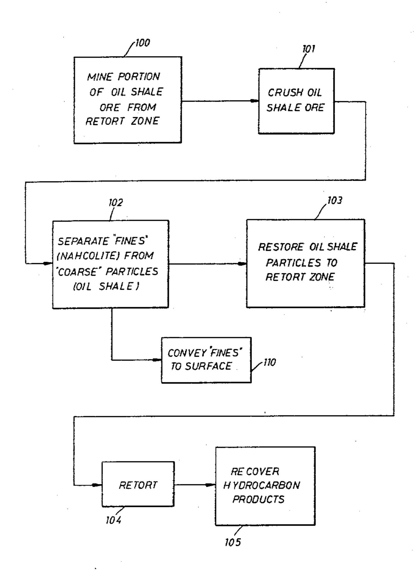
F1G. 1 MINE PORTION OF OIL SHALE CRUSH OIL ORE FROM SHALE ORE RETORT ZONE 103 102 SEPARATE "FINES" RESTORE OIL SHALE (NAHCOLITE) FROM PARTICLES TO "COARSE" PARTICLES RETORT ZONE (OIL SHALE) CONVEY FINES" TO SURFACE
