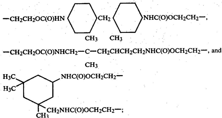
ureadiacetoacetamide copolymers, that is, copolymers prepared by the reaction of at least one polyfunctional acrylate with at least one ureadiacetoacetamide in the presence of a catalyst capable of promoting the reaction between the polyfunctional acrylate and the ureadiacetoacetamide. These acrylate-
