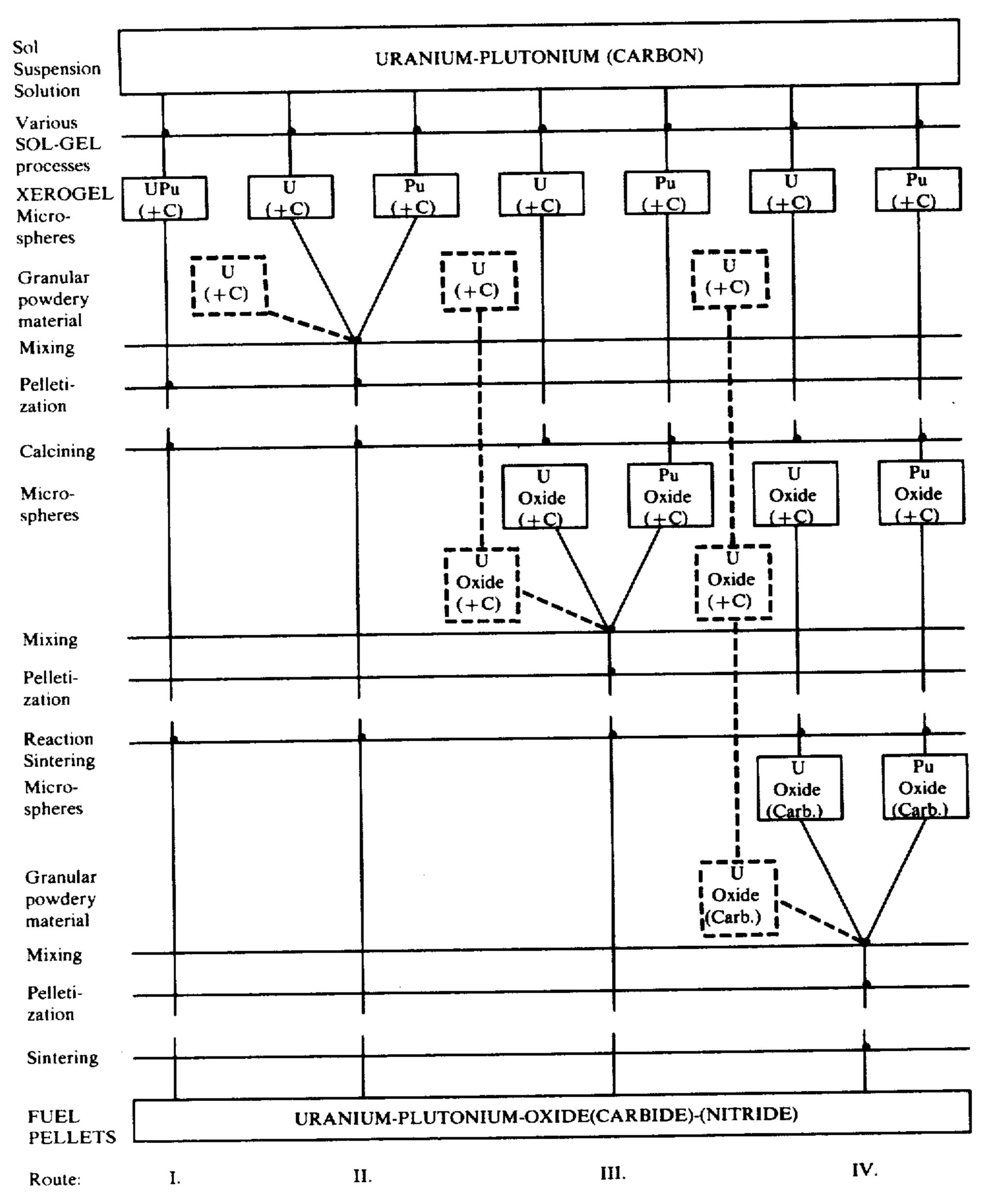
Route I One starts with a uranium-plutonium xerogel which contains finely divided carbon for the production of carbide pellets in the microspheres.
