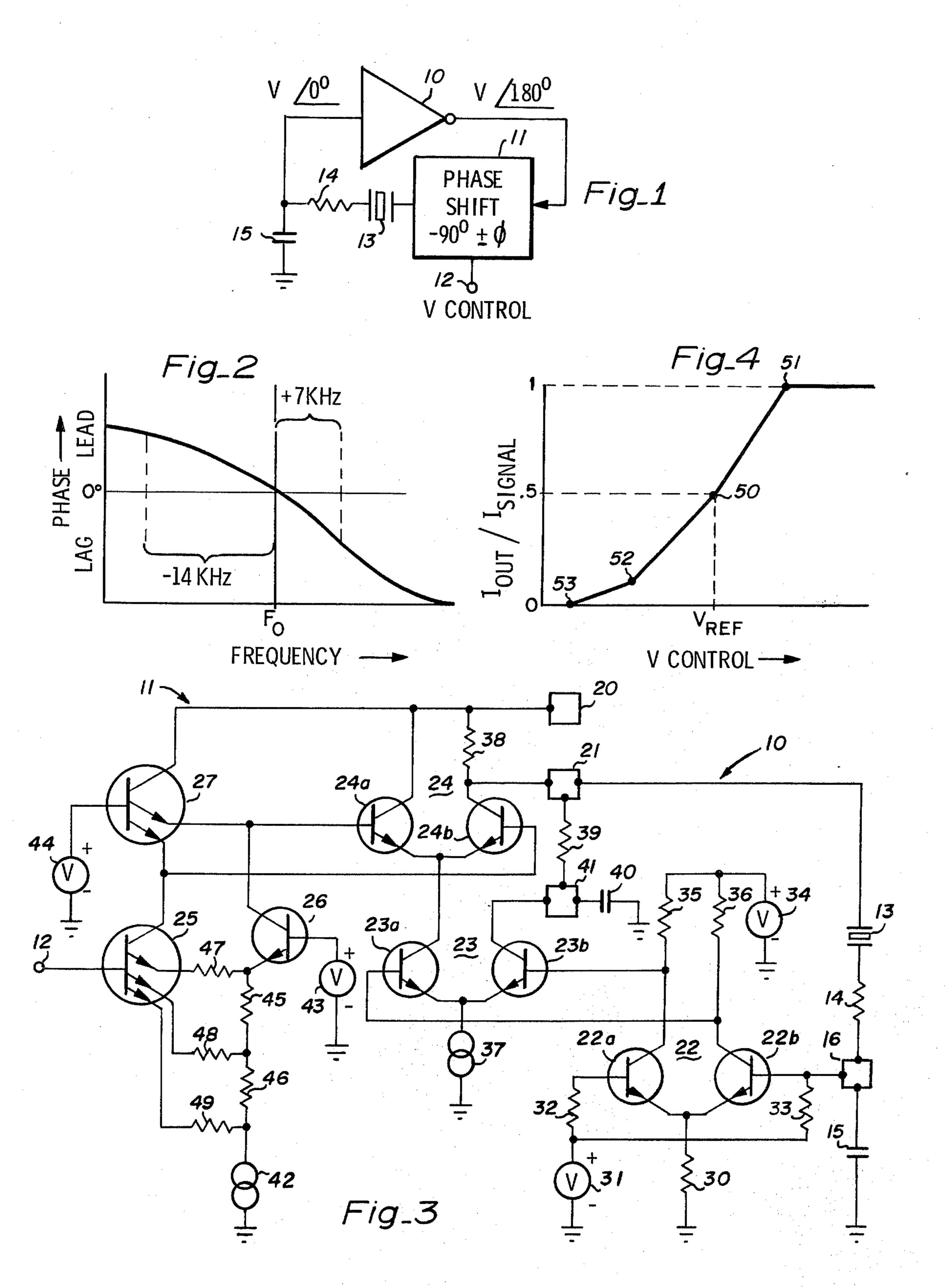
can be compensated so that the overall voltage versus frequency response is linear.
