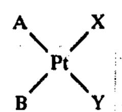
in which X and Y are the same or different ligands selected from sulphate, phosphate, nitrate, carboxylate, halogen-substituted carboxylate and water and A and B are the same or different branched chain aliphatic amines co-ordinated to the Pt through their N atoms, such that the platinum is present as Pt<sup>2+</sup>.
