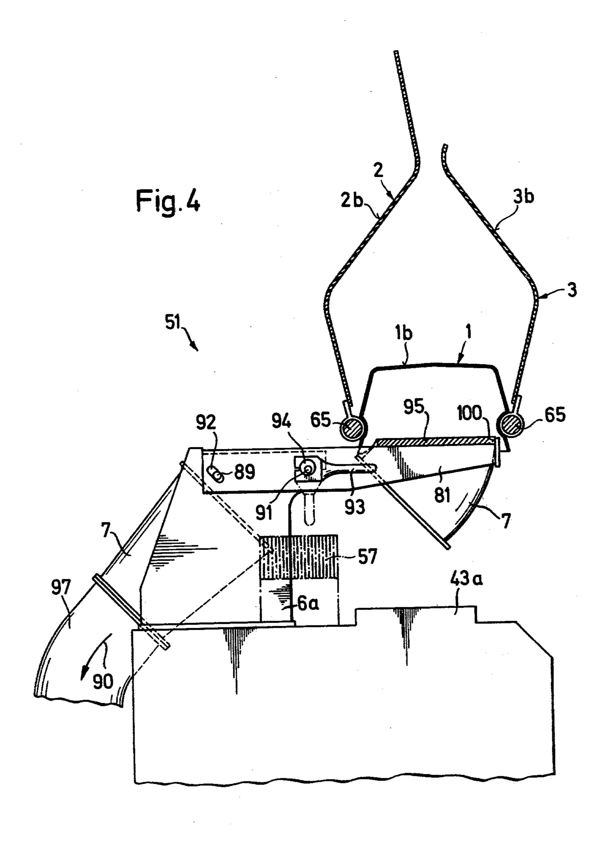
WEAVING MACHINE HAVING AN AIR DUCT FOR CLEANING PURPOSES
