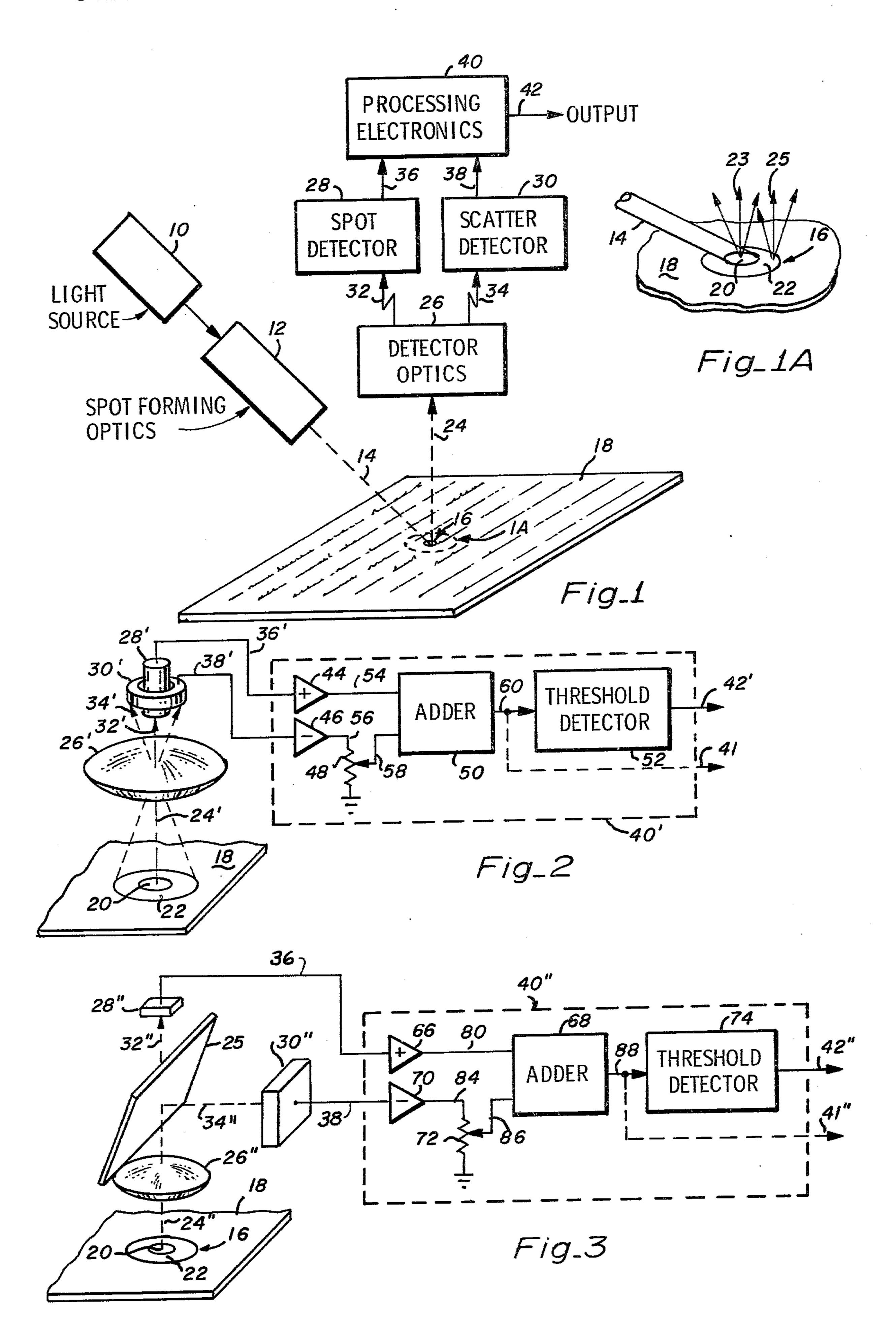
compensating for the effects of surface light scatter in an optical reflective scanning system.
