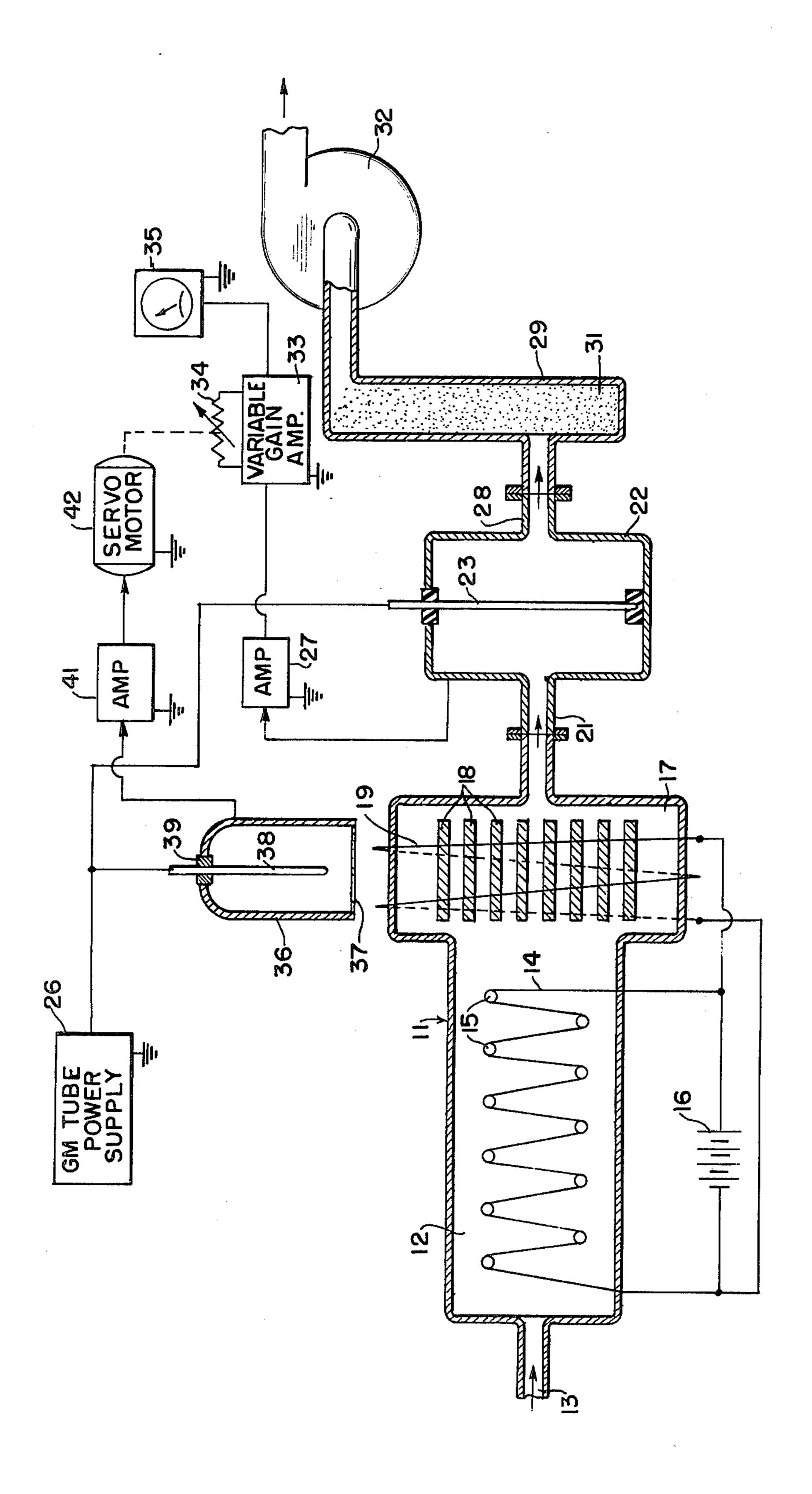
This invention relates to an apparatus and method for 5 detecting gases containing specific halogen containing compounds.
