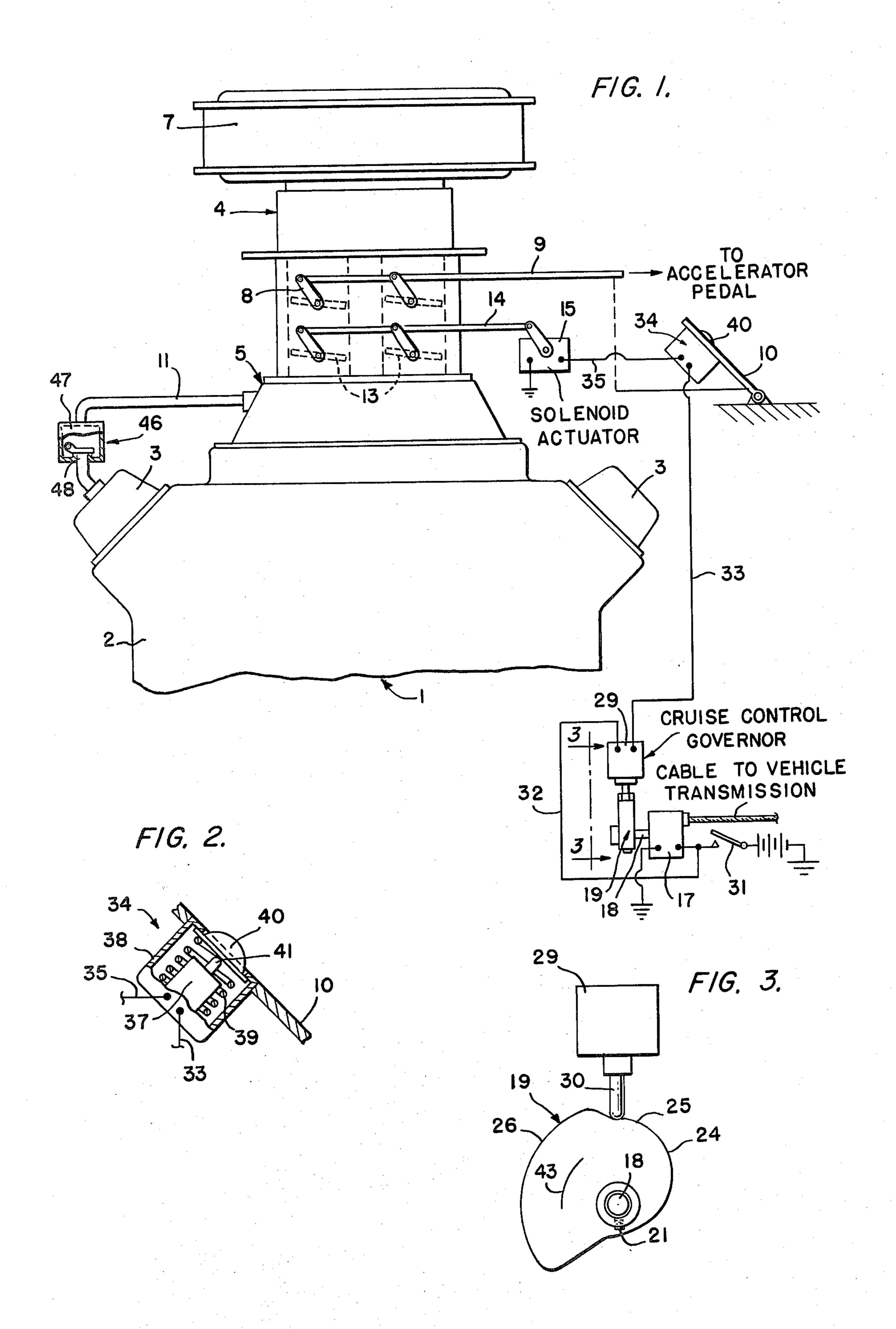
FIG. 2 is a cross sectional view of the switch means located on the accelerator pedal.
