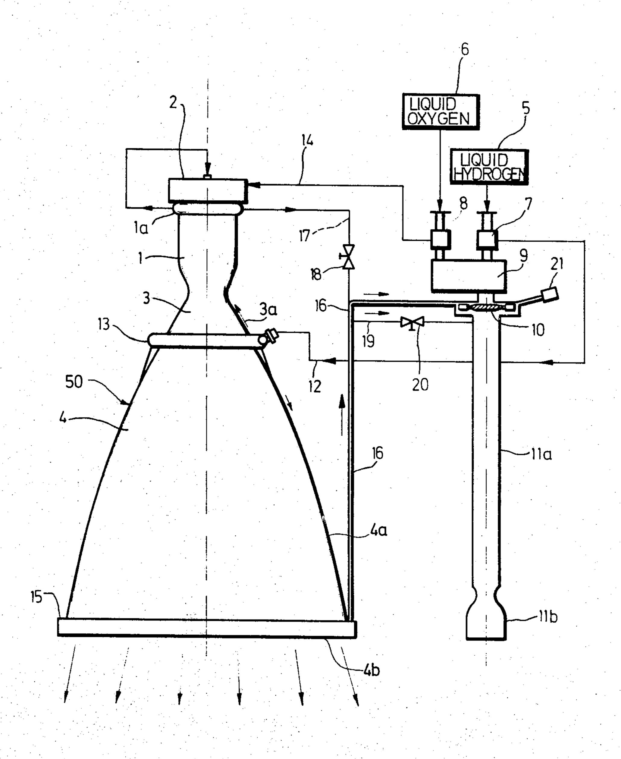
LIQUID FUEL ROCKET ENGINE HAVING A PROPELLANT COMPONENT PUMP TURBINE WITH A SECONDARY THRUST DISCHARGE AND TO A METHOD OF OPERATING A LIQUID FUEL 5 ROCKET ENGINE
