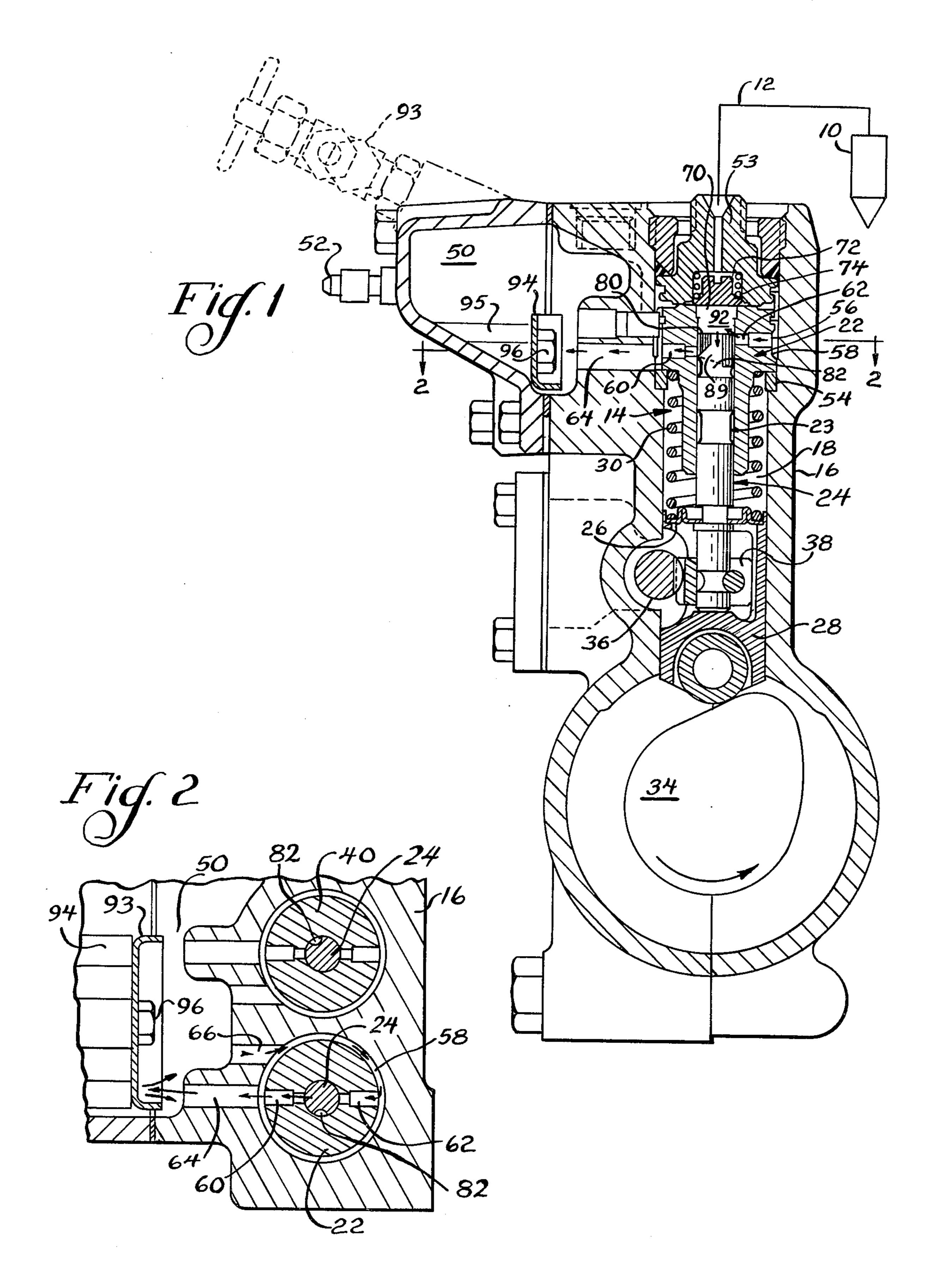
FIG. 2 is a horizontal sectional view of the fuel pump
