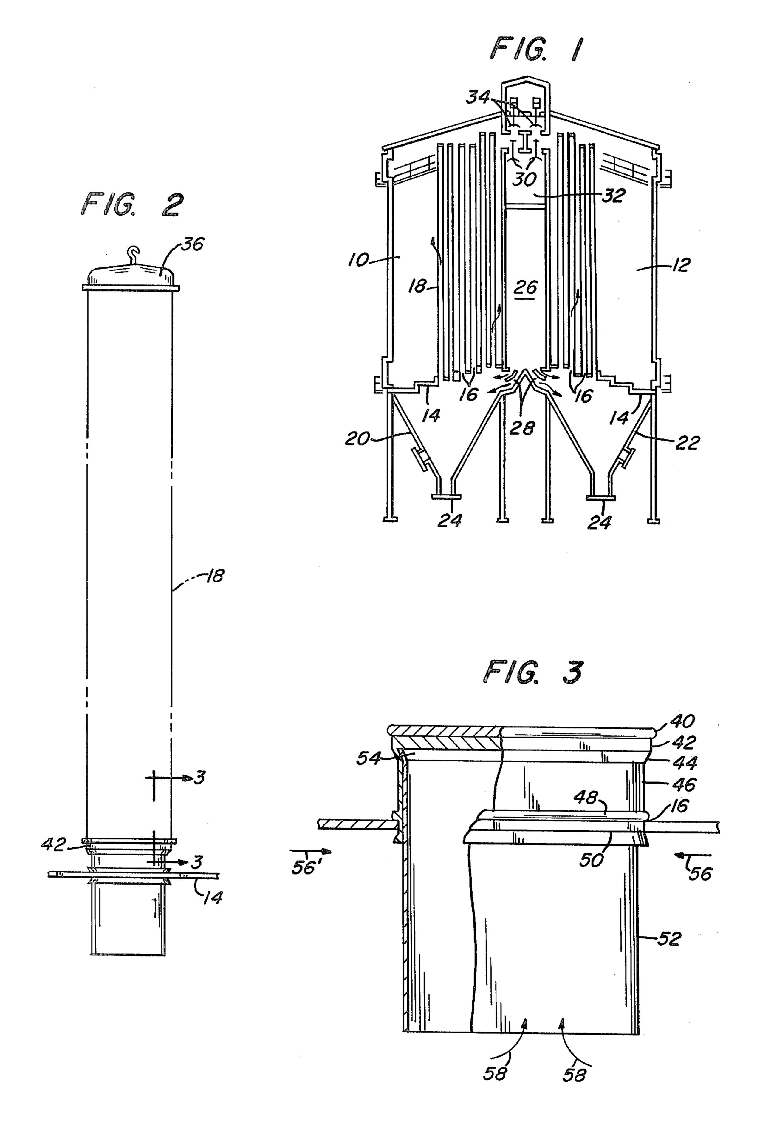
FIG. 1 is a schematic cross-sectional view of a baghouse with which the present invention may be used;
