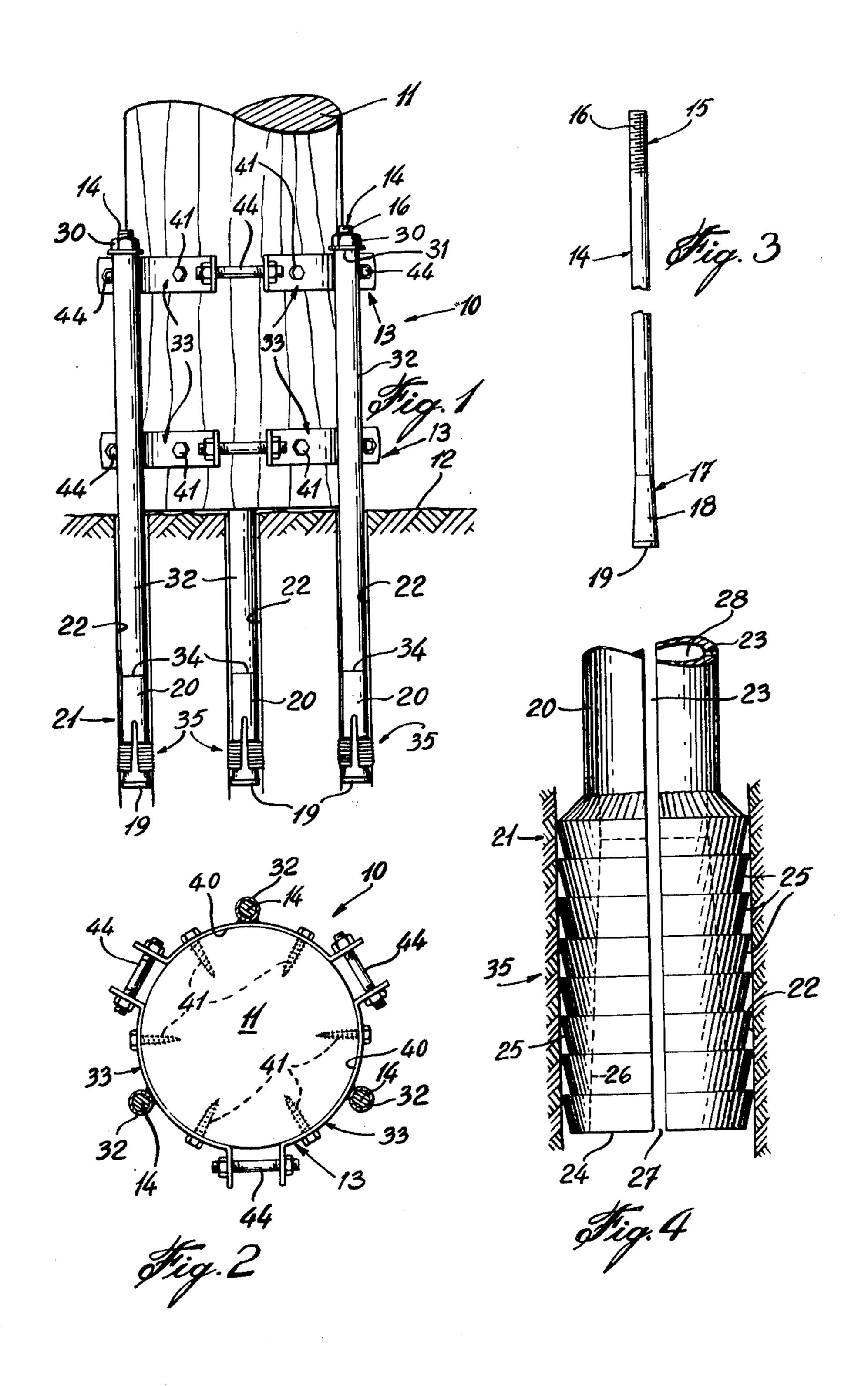
such as rock or concrete. The bracket 10 comprises essentially a clamp device 13 which is securable to the article 11 and at least two anchor rods 14, three being
