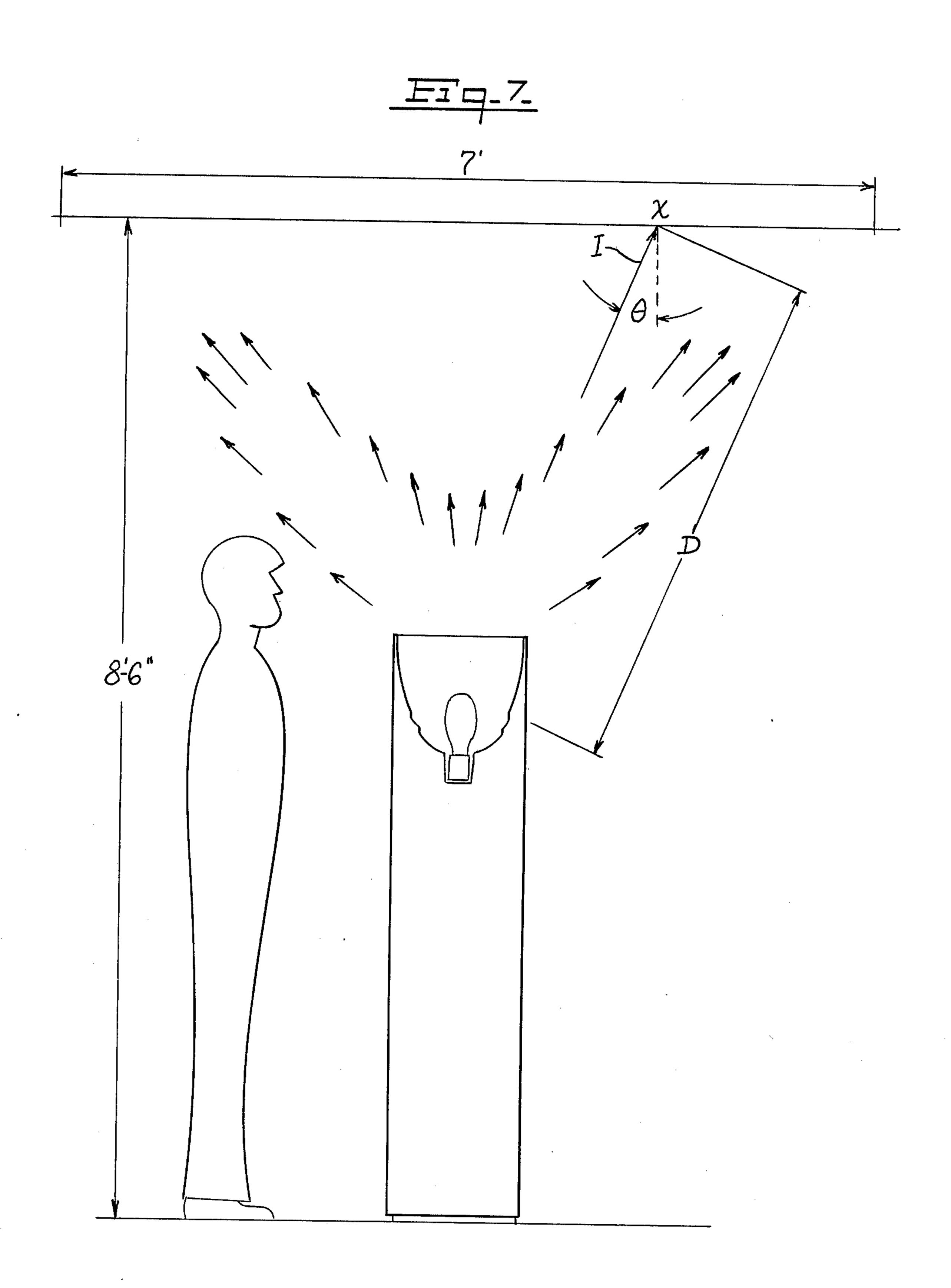
This invention relates to luminaires, of square or circular cross section, wherein the reflecting surfaces include a combination of one parabolic element and 5 three elliptical elements, so proportioned and oriented as to produce very uniform distribution of light, particu-
