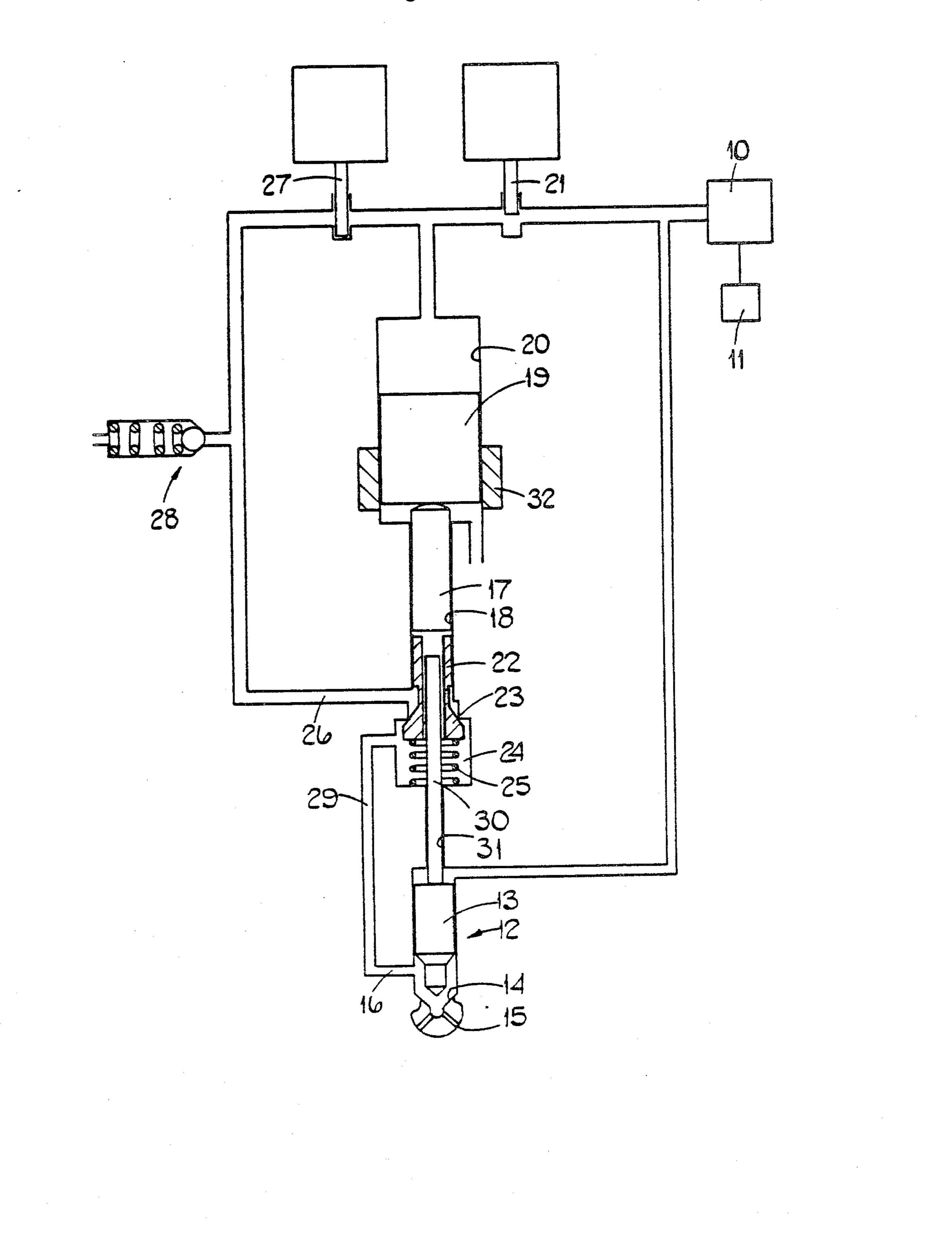
on the valve member 13 to lift it from the seating thereby to allow fuel flow through the orifices 15.
