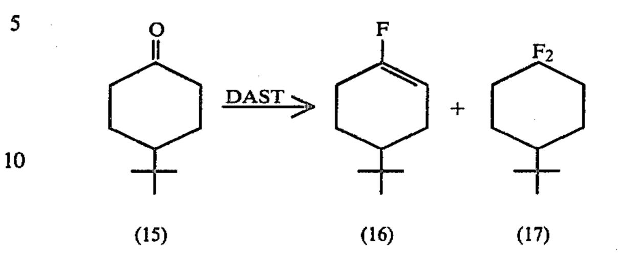
A. A 20.0 g amount of 4-t-butylcyclohexanone was dissolved in 230 ml of glyme at room temperature in a dried Teflon ® bottle under N<sub>2</sub>, with stirring. Five milliliters of 20% fuming sulfuric acid was added and the mixture was stirred for 5 min. Forty milliliters (44.4 g) of diethylaminosulfur trifluoride was added. The resultant mixture was stirred at ambient temperature under N<sub>2</sub> for 24 hours.
