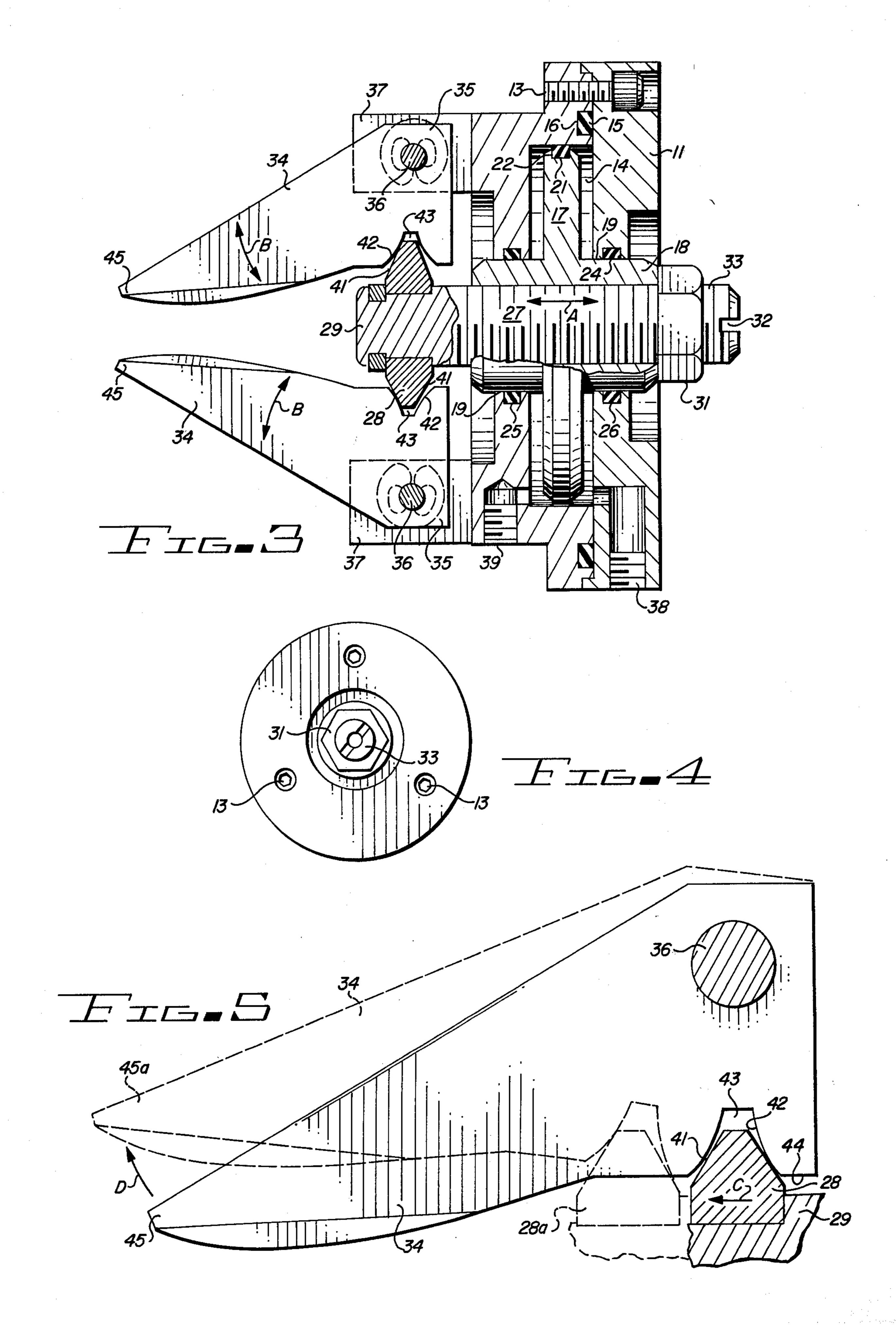
member and the lever fingers utilizes "rolling" contact between the mating surfaces of the mechanism.
