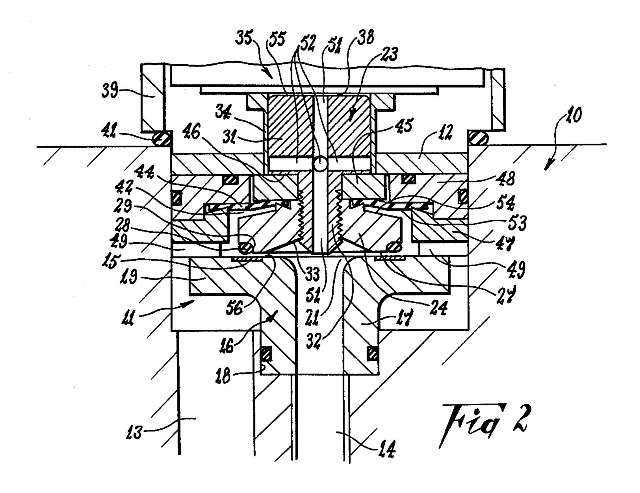
This invention relates to valves of the kind used in controlling a jet of fluid of variable duration. Such 5 valves are commonly used in ore sorting and it will be convenient to hereinafter describe the invention in relation to that example application.
