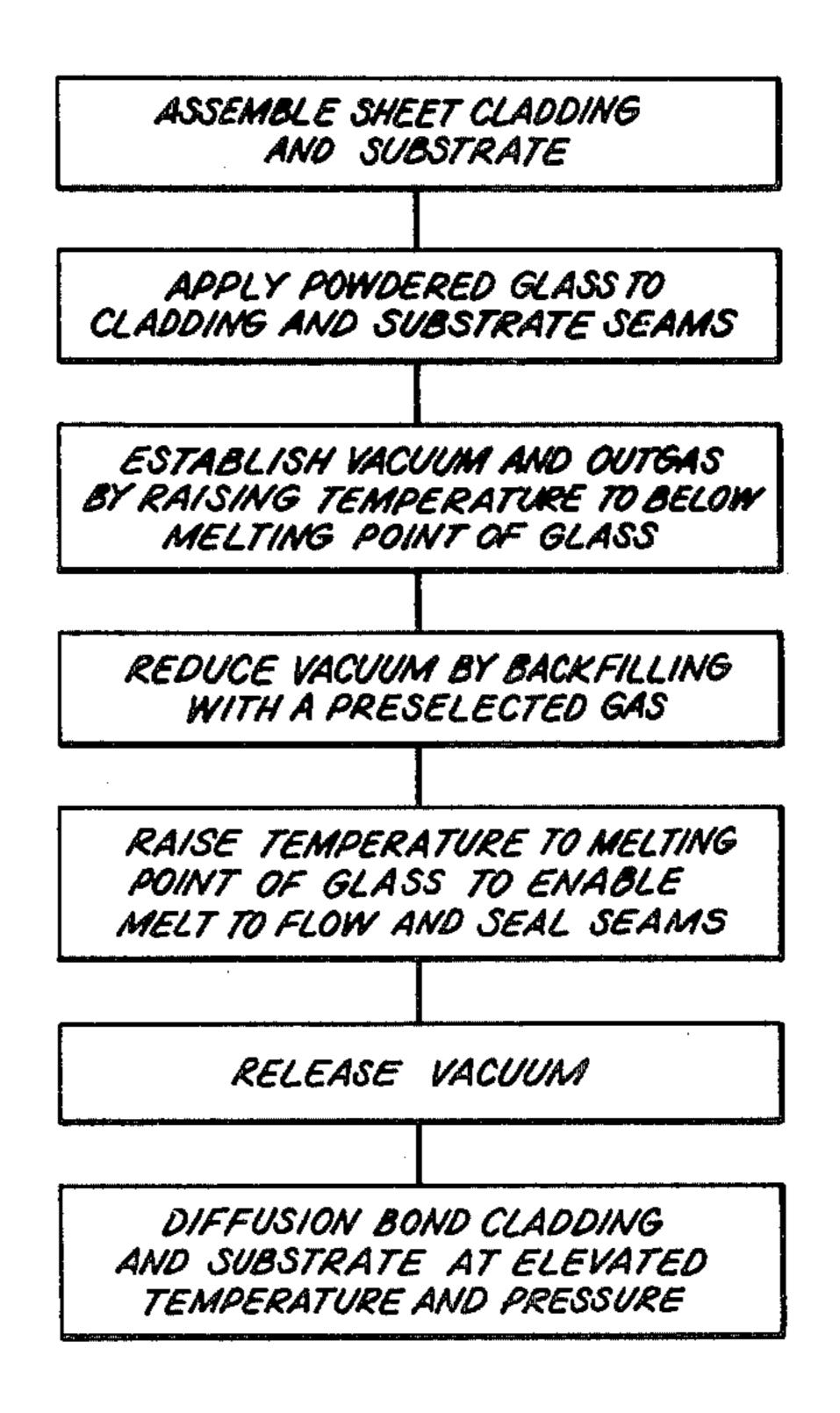
ASSEMBLE SHEET CLADDING AND SUBSTRATE
