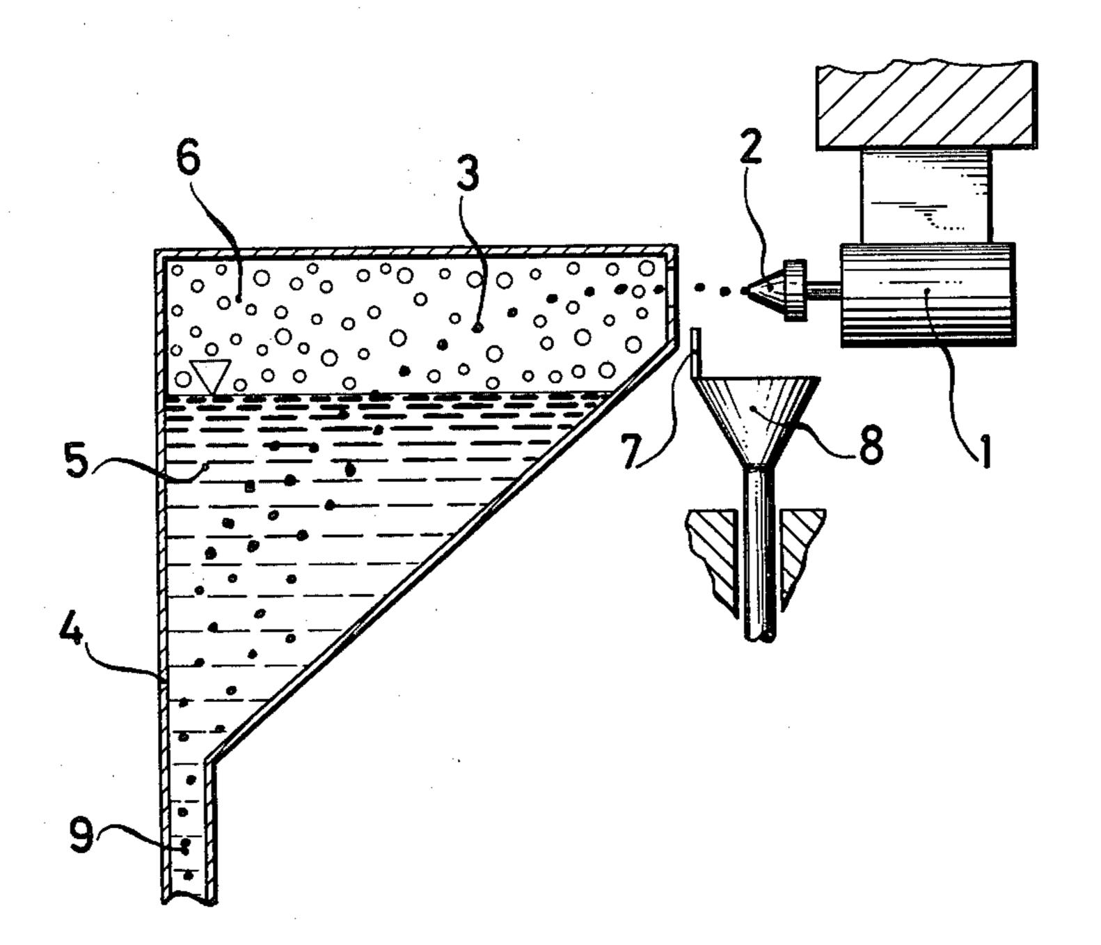
ARRANGEMENT FOR THE PRODUCTION OF SPHERICAL PARTICLES FROM DROPS OF AQUEOUS NITRATE SOLUTIONS OF URANIUM, PLUTONIUM OR THORIUM, OR MIXTURES OF THESE MATERIALS FOR FUEL AND BREEDER ELEMENTS FOR NUCLEAR REACTORS
