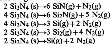
45 From this reaction, it would be expected that densification would be enhanced by sintering in an inert environment under high pressure and, indeed, such has been the practice of the prior art. However, sintering in a high pressure environment requires bulky and expensive equipment and exposes workers to possible hazards from explosion and the like.
