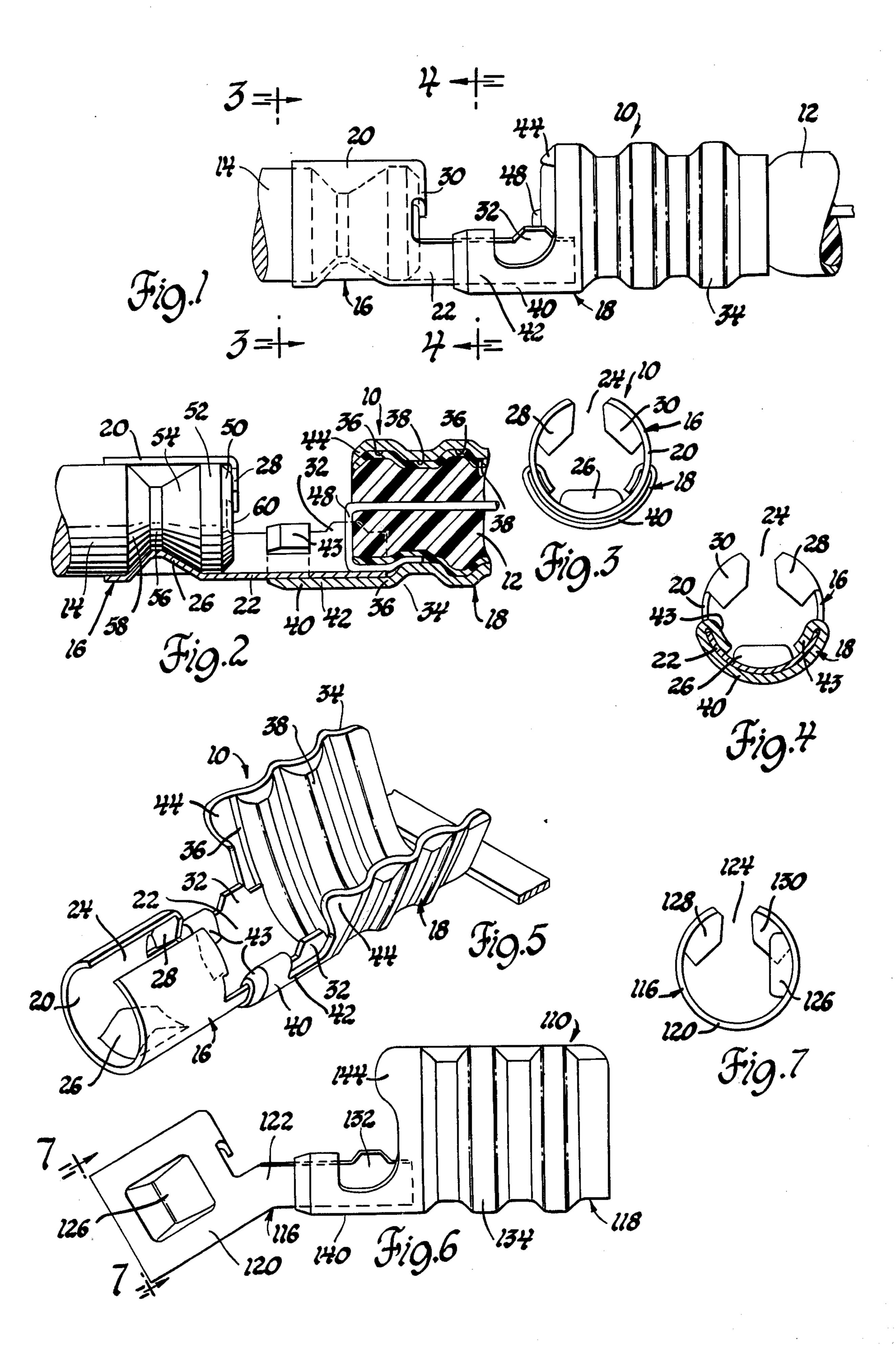
pered steel for an improved electrical connection under conditions of vibration.
