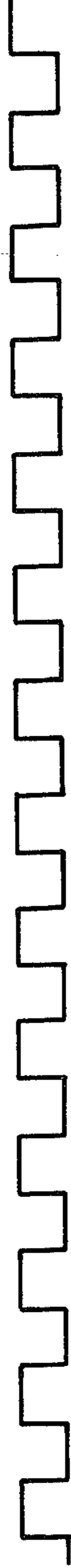
FIG. 4D INVERTED CLOCK PULSES
