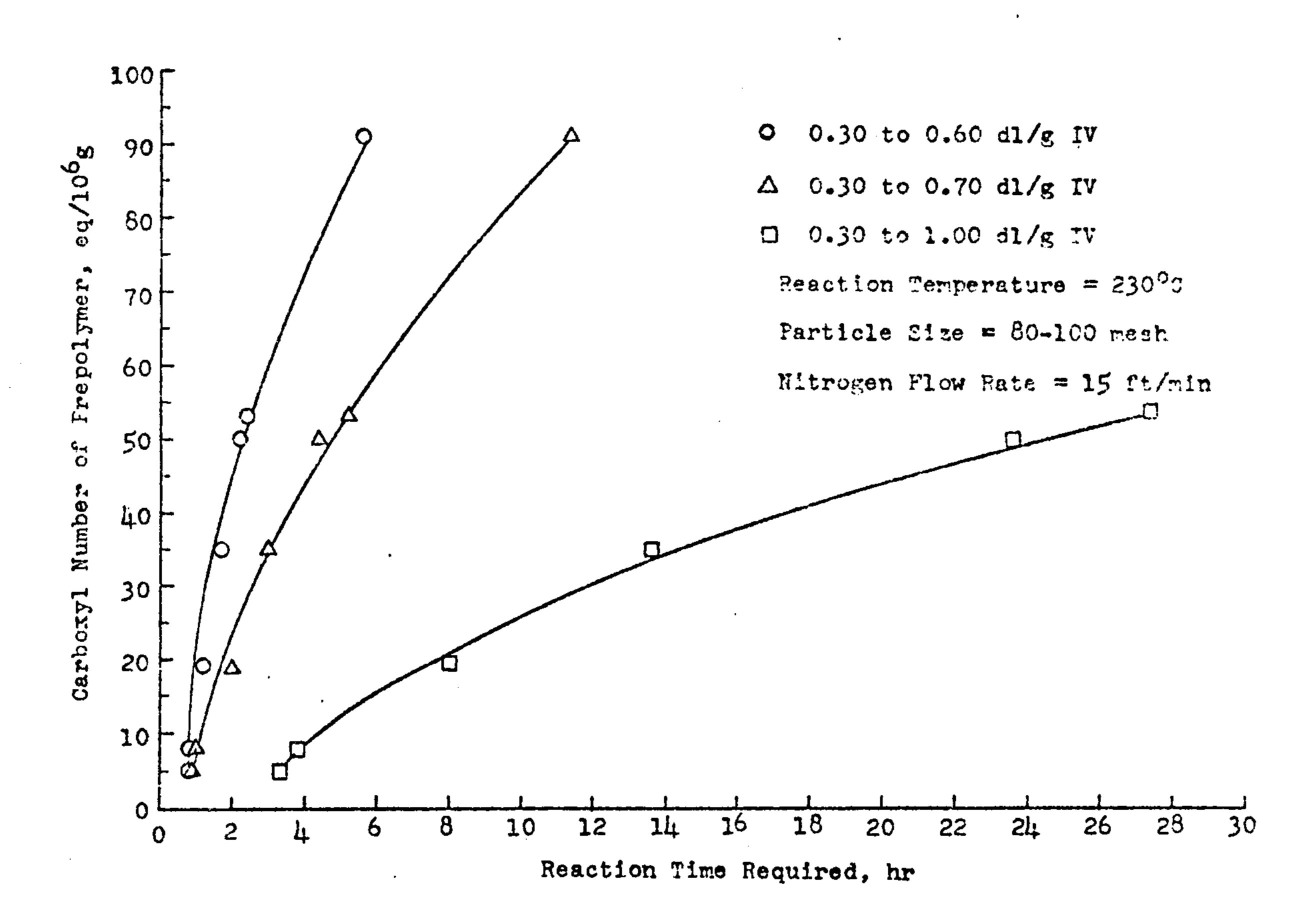
Thus, it can be seen that the stability and color clarity of the polyester polymer is improved by a reaction process which utilizes a two-stage polymerization. To achieve the maximum rate for this polymerization, prepolymers having minimal carboxyl content, which requires minimal catalyst levelsn, are produced.
