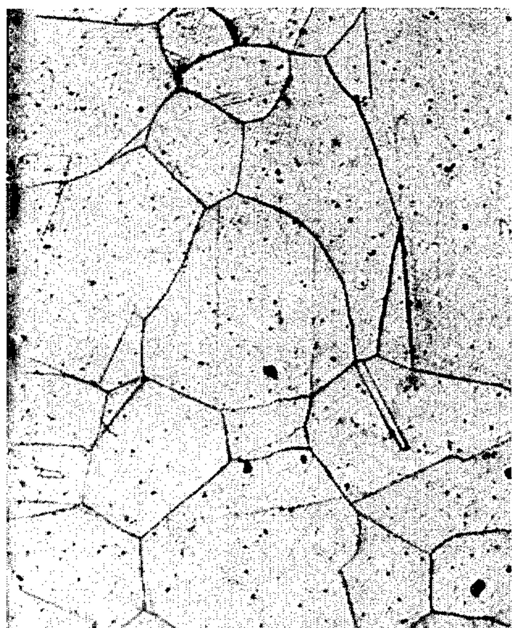
FIG. 6 10% REDUCTION, SURFACE. HEATED TO 2300° FOR ROLLING
