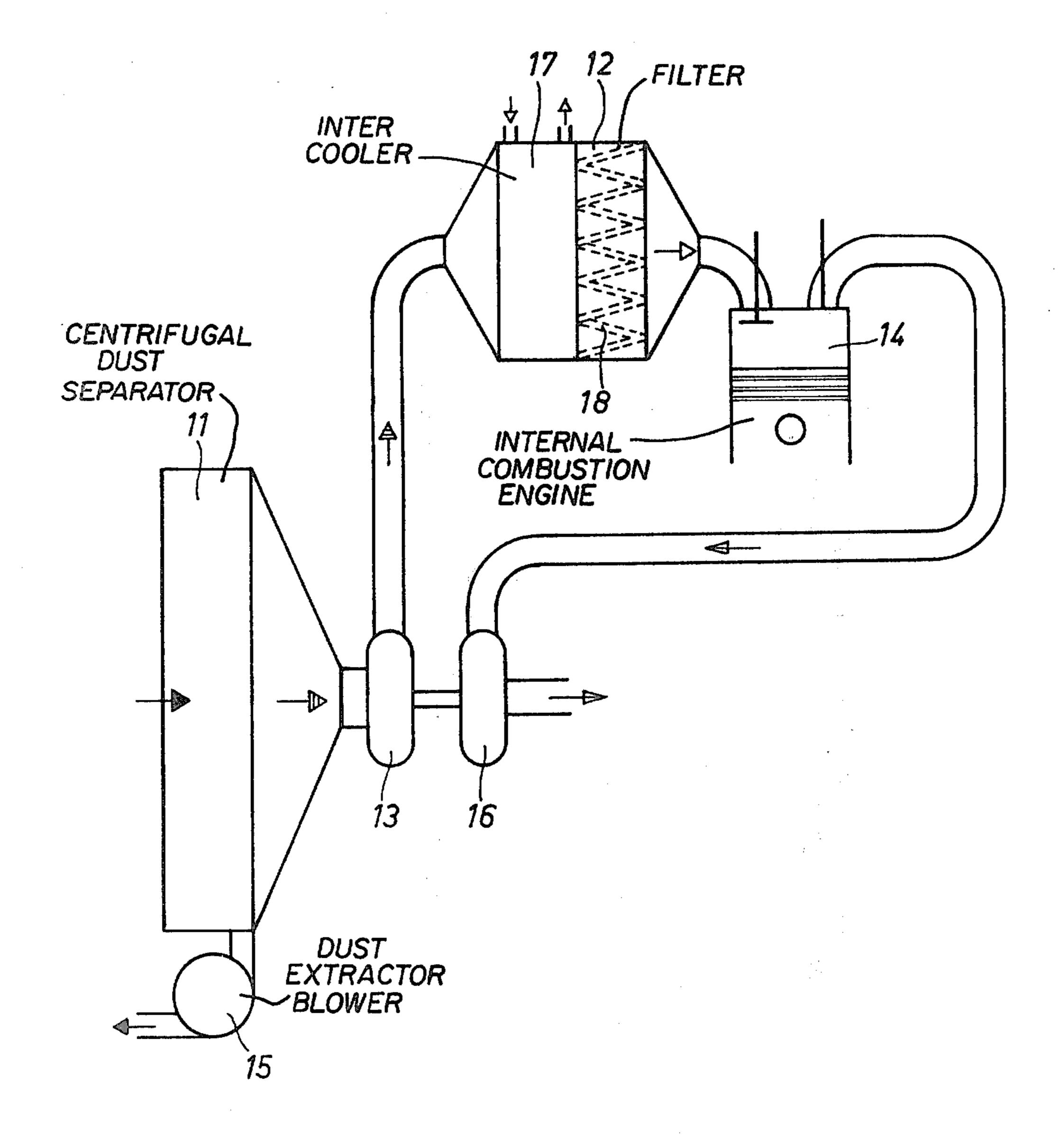
tion to the same air volume flow, a filter insert of paper felt results in a smaller filter structural size of the dry air filter than with the use of the temperature-resistant filter material.
