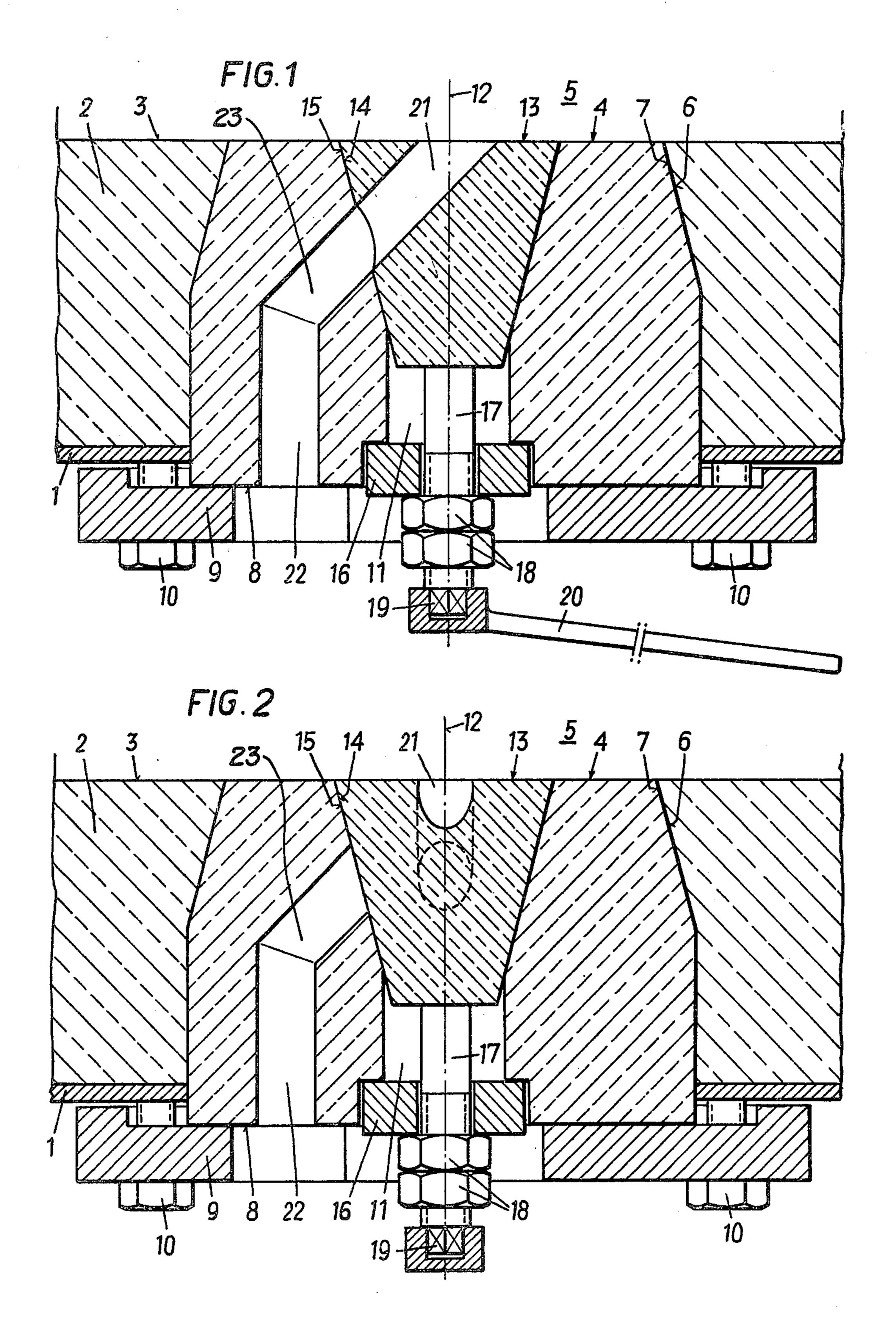
Suitably, the closure block is provided with an operating extension projecting to the outer side of the vessel.
