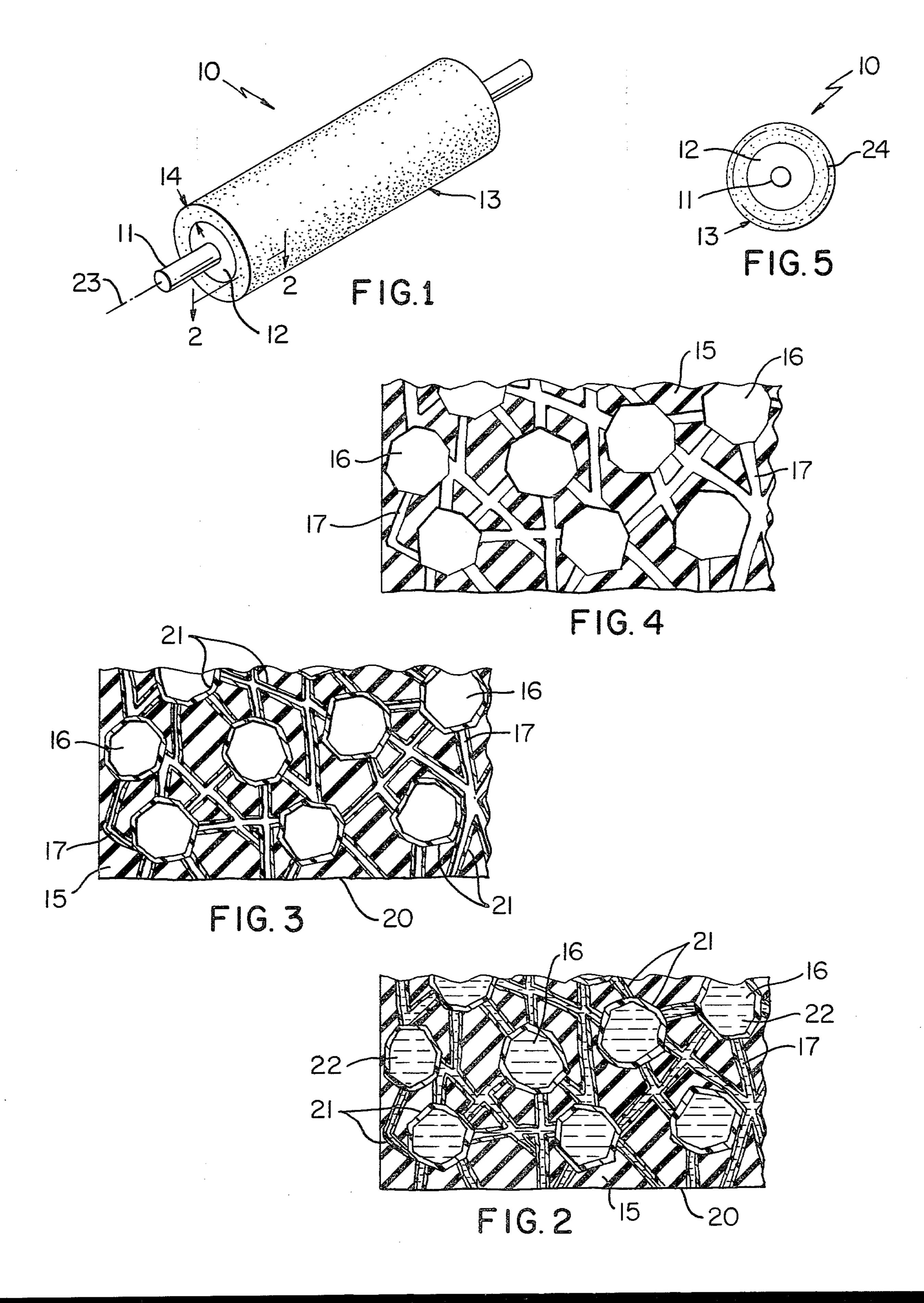
FIG. 3 is a view similar to FIG. 2 minus the ink formulation to highlight the lining of the thermally expandable and contractible plastic material in the outer
