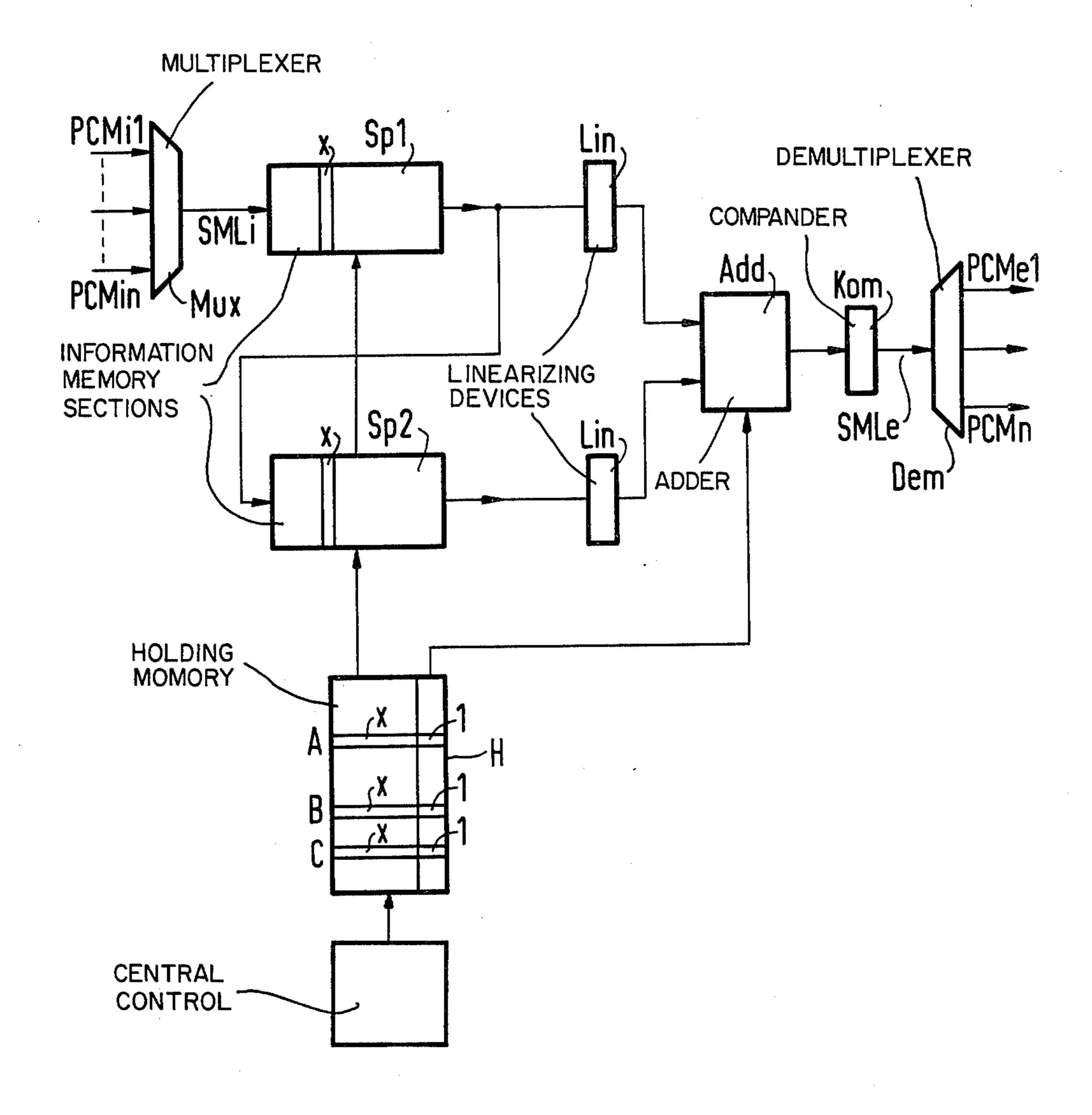
CIRCUIT ARRANGEMENT AND PROCESS FOR PRODUCING CONFERENCE CONNECTIONS BETWEEN THREE CONFERENCE PARTIES IN A PCM TIME MULTIPLEX SWITCHING SYSTEM
