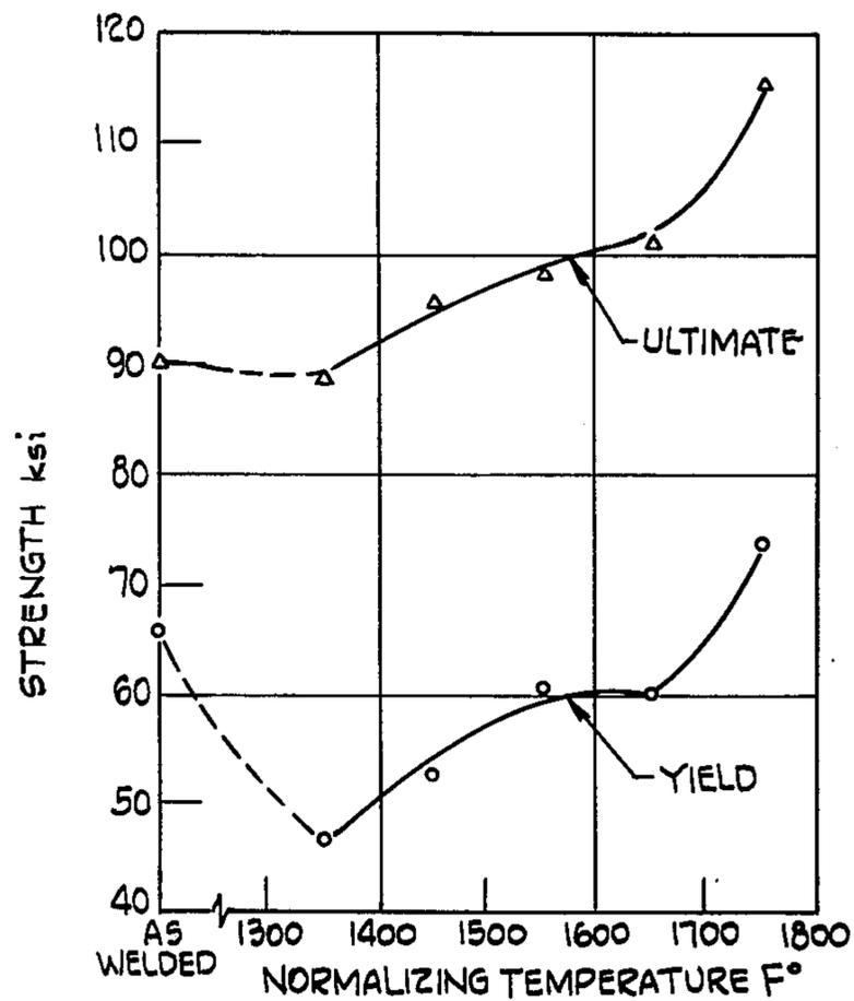
CHROMIUM STEEL, AS WELDED PIPE, 0.380-INCH WALL THICKNESS
