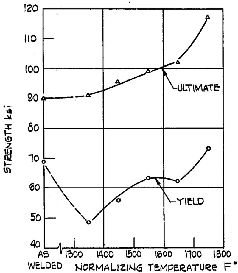
CHROMIUM STEEL, AS WELDED PIPE, 0.480 INCH WALL THICKNESS
