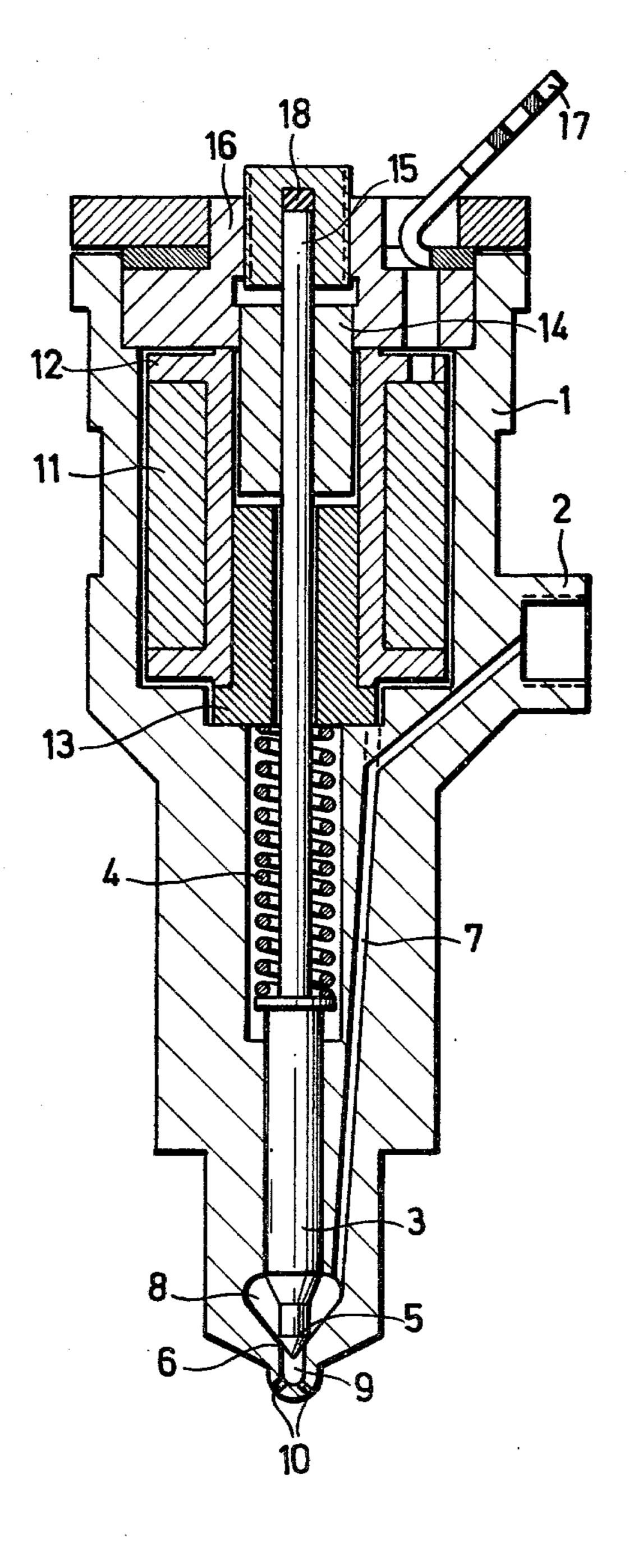
The present invention relates to a fuel injector for internal combustion engines, and comprises a controlla- 5 ble fuel injection pump and a fuel injection valve, which has a spring-loaded valve needle which opens counter to the direction of flow of the fuel, and which is acted upon by an additional closing force during closing.
