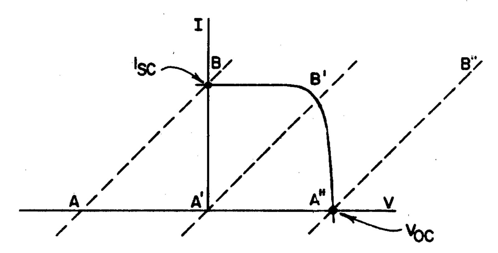
Voc = OPEN CIRCUIT (NO LOAD CURRENT)
