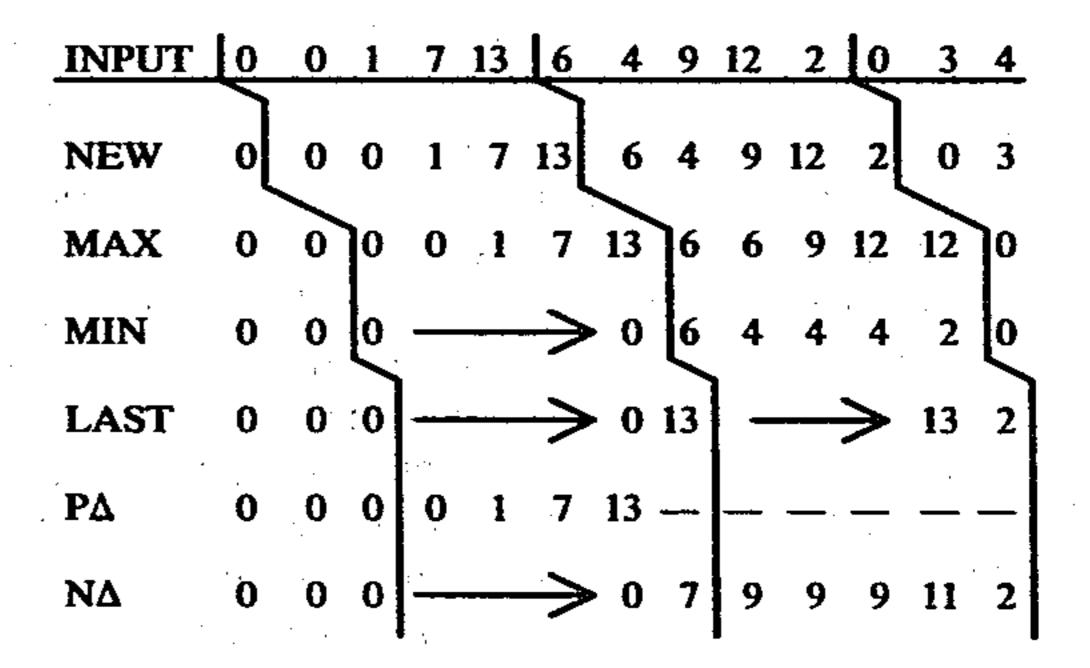
A video signal is sampled through two sampling intervals during which five samples per interval are taken and converted to digital form by an analog-to-digital These samples are entered into the new data buffer register 10 at the end of each sample clock period as represented by the second row of digits. (For conve-
