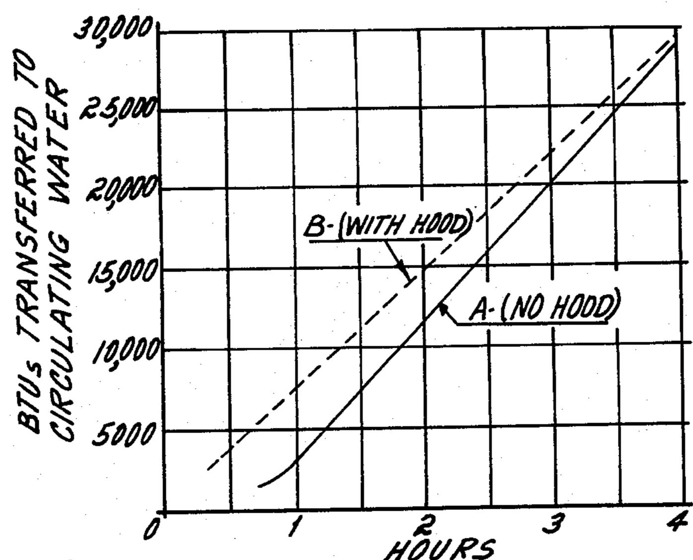
HOURS ATES OF HEAT TRANSFER TO WATER IN COIL
