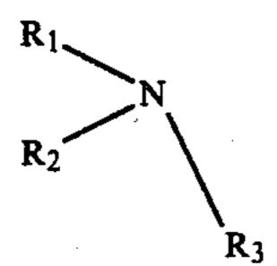
wherein R<sub>1</sub>, R<sub>2</sub>, and R<sub>3</sub> can each be alkyl containing from 1 to 8 carbon atoms. Thus, for example, the tertiary amine can be a trialkyl amine such as trimethylamine, triethylamine, tri-isopropylamine, tri-n-propylamine, tri-isobutylamine, tri-n-butylamine and the like. In addition, tertiary amines such as pyridine, and thos containing diamine groups such as N,N,N',N'-tetramethylethylene diamine (TMEDA) can also be utilized.
