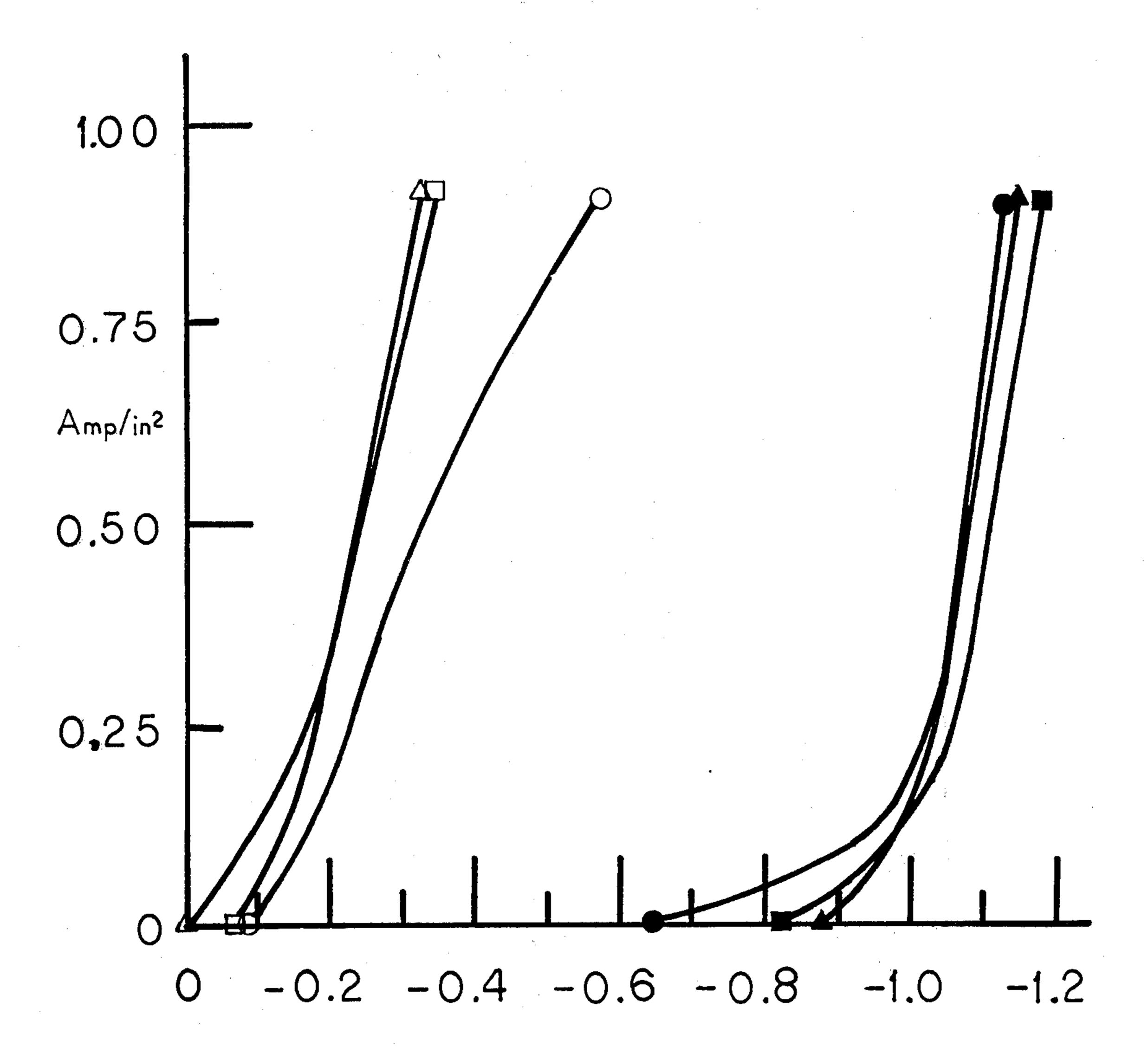
Cathode Voltage vs. Ag/AgCI (taken on a set of three 10 wt. % Pt compacts, with open figures denoting oxygen and solid figures denoting nitrogen)
