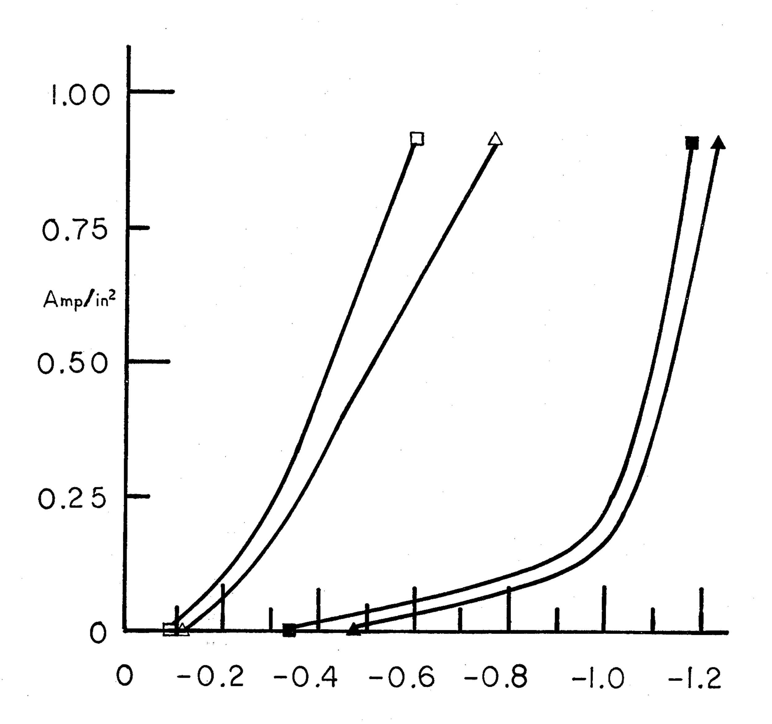
Cathode Voltage vs. Ag/AgCl (taken on a set of two 10 wt. % Ag compacts, with open figures denoting oxygen and closed figures denoting nitrogen)
