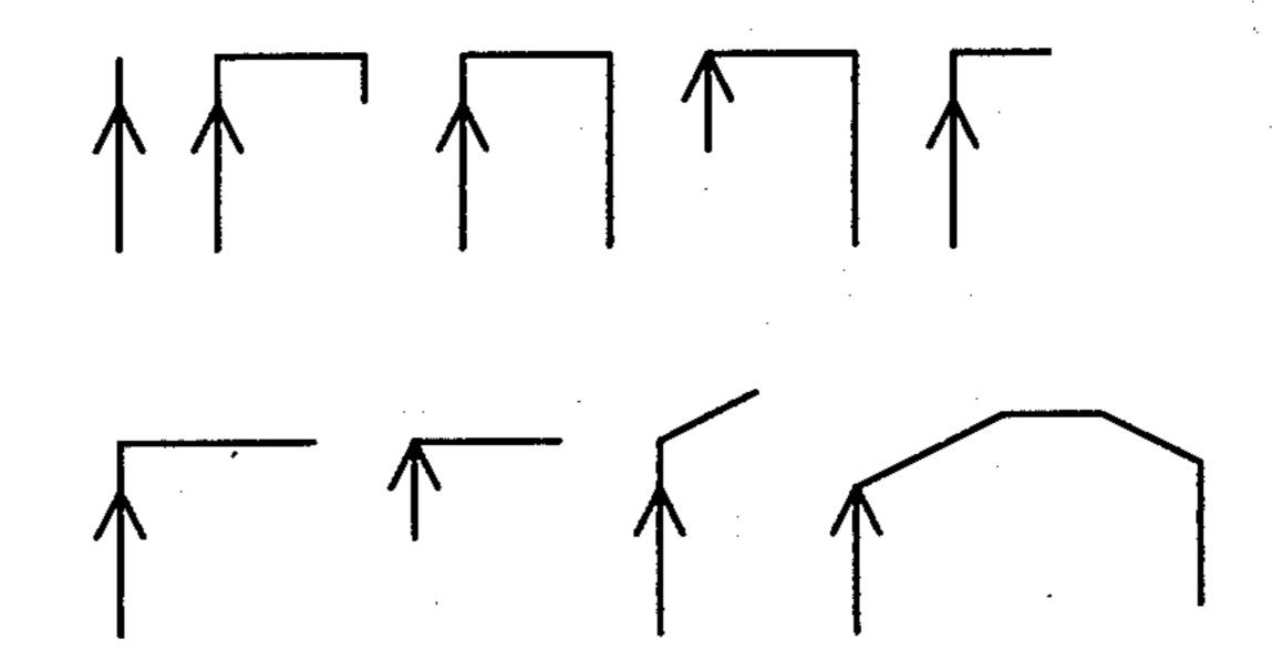
The illustrated nine shapes, along with the conjugates of the second through ninth shapes, provide a set of seventeen selected canonic shapes which are later matched against the character curve segments of the character being scanned so that a "best match" can be determined and used in the recognition process of the present invention.
