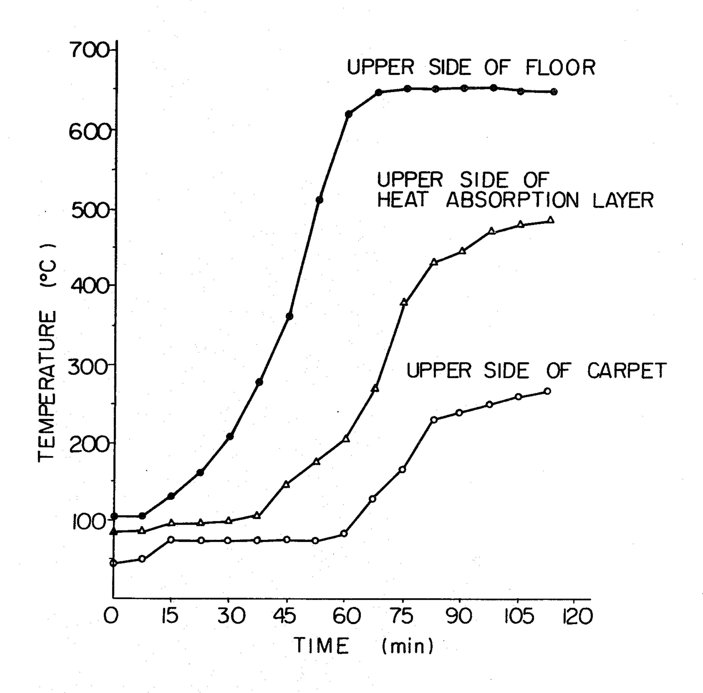
HEAT ABSORPTION MEANS OPERATIVE AT PRESCRIBED TEMPERATURE FOR SUPPRESSION OF HEAT TRANSFER FROM ABNORMALLY HEATED AUTOMOTIVE EXHAUST SYSTEM TO ARTICLE ON BOARD
