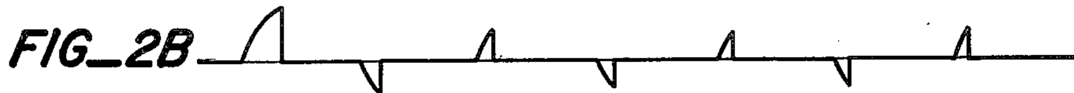
SUPPLY WINDING CURRENT AT W1
