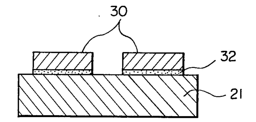
PROCESS FOR MANUFACTURING A VAPOR PHASE EPITAXIAL WAFER OF COMPOUND SEMICONDUCTOR WITHOUT CAUSING BREAKING OF WAFER BY UTILIZING A PRE-COATING OF CARBONACEOUS POWDER
