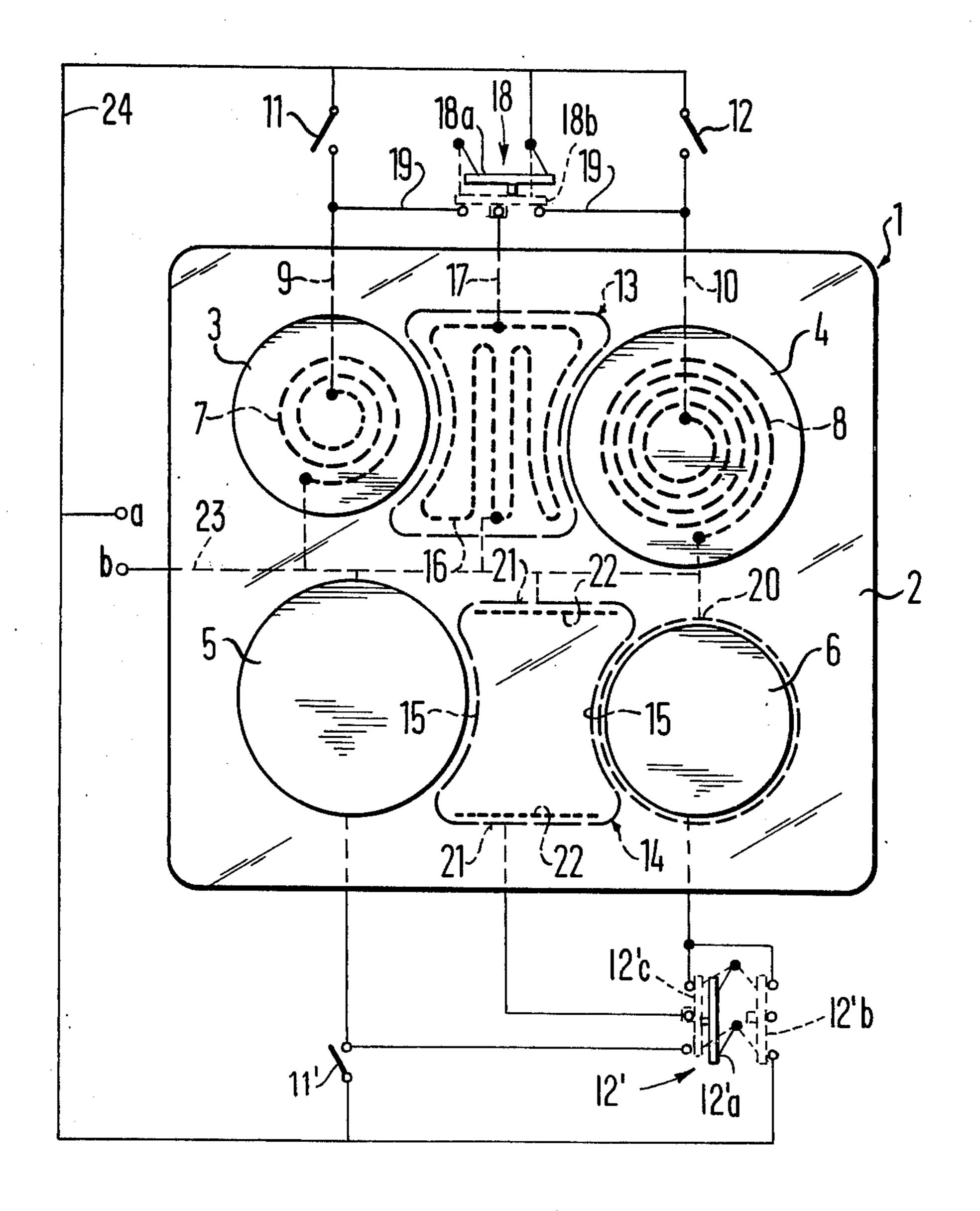
The invention relates to a stove or range top with a support plate having several main cooking stations which are located spaced from one another and are switchable on and off individually by main switching means associated with the cooking stations.
