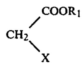
wherein R<sub>1</sub> represents vinyl, allyl or methallyl, and X represents cyano or COOR<sub>2</sub> in which R<sub>2</sub> represents methyl, ethyl or propyl, in an aqueous medium and in the presence of a copolymerization catalyst at a temperature of 5°-95° C. for 30-120 minutes, the acrylic ester component being added to the copolymerization system in a dropwise manner, and (2) vulcanizing the resultant copolymer with a vulcanizing agent of the thiuram series.
