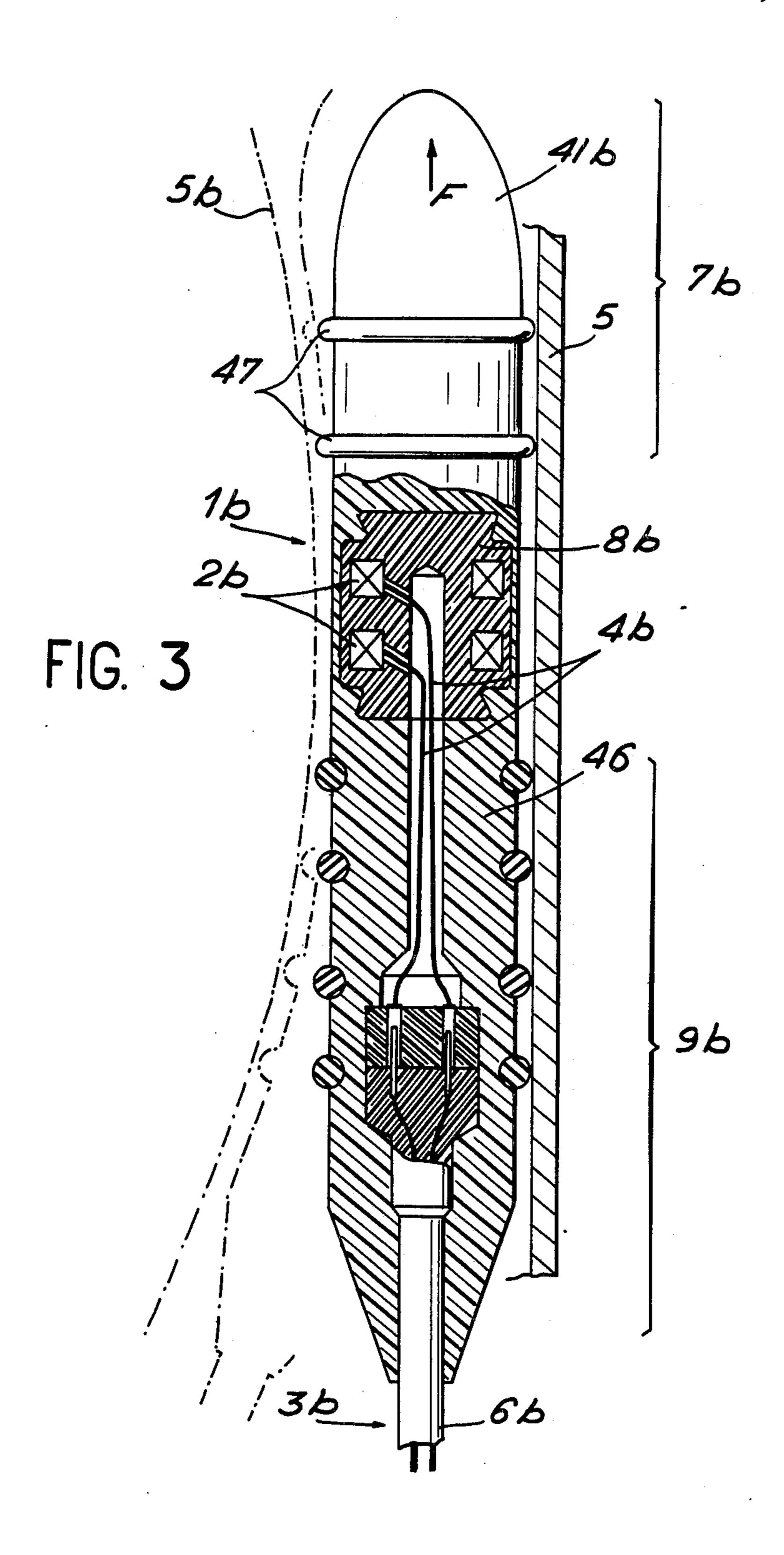
However, when the tubes to be tested have small internal diameters with relatively substantial lengths and are bent at least locally, probes of the usual types do not prove wholly satisfactory, especially at the time of the passage of elbowed zones, ovalized zones or even
