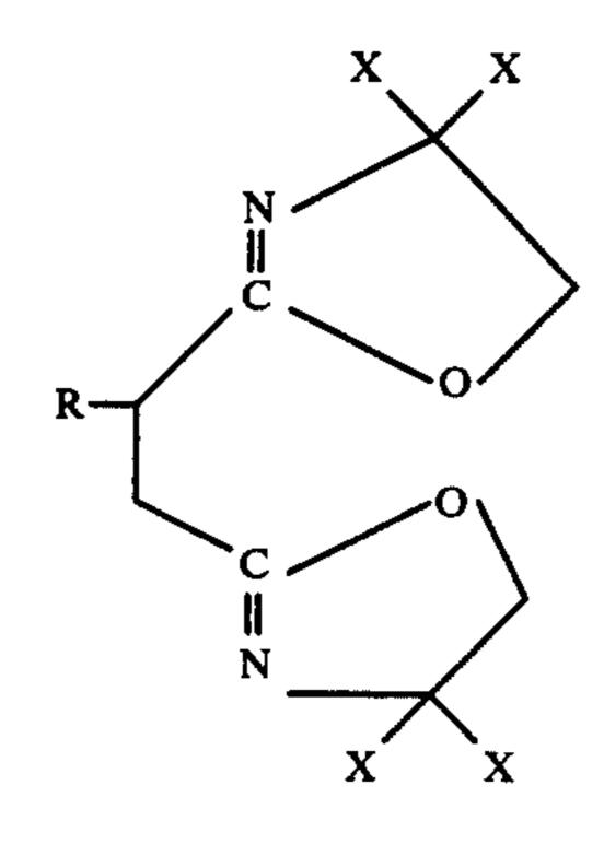
wherein X is alkyl or hydroxy alkyl, said alkyl groups having 1 to 3 carbon atoms, and at least one of said X is a hydroxy alkyl group of the structure  $-(CH_2)_nOH$  where n is 1 to 3; at a temperature in the range of about 140° to 240° C. for about  $\frac{1}{2}$  to 24 hours with the removal of about three molar proportions of water to thereby produce said bis-oxazoline having the structure
