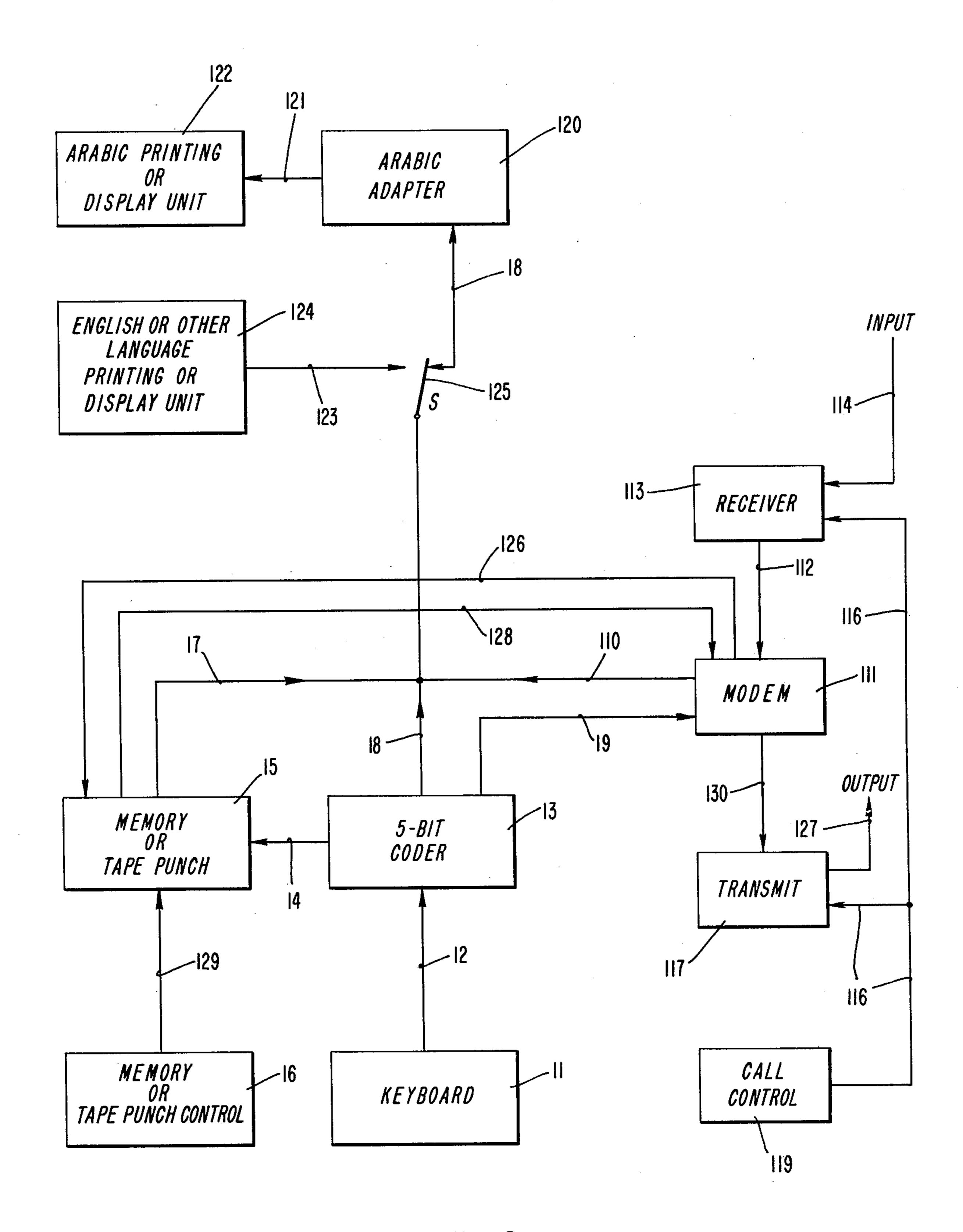
5-BIT BINARY BAUDOT CODED ARABIC
