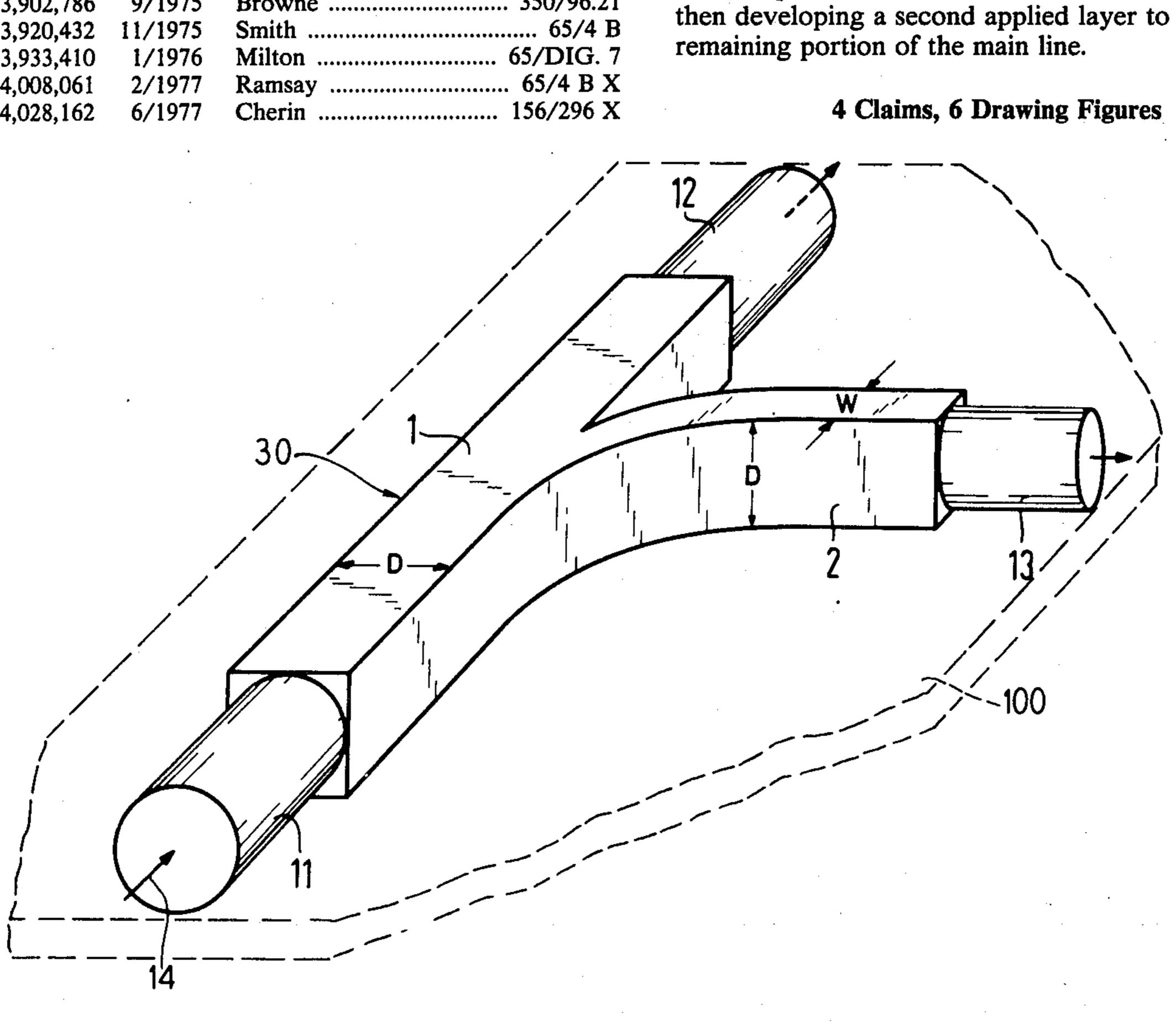
METHOD FOR MAKING OUTPUT/INPUT COUPLER FOR MULTI-MODE GLASS **FIBERS**
