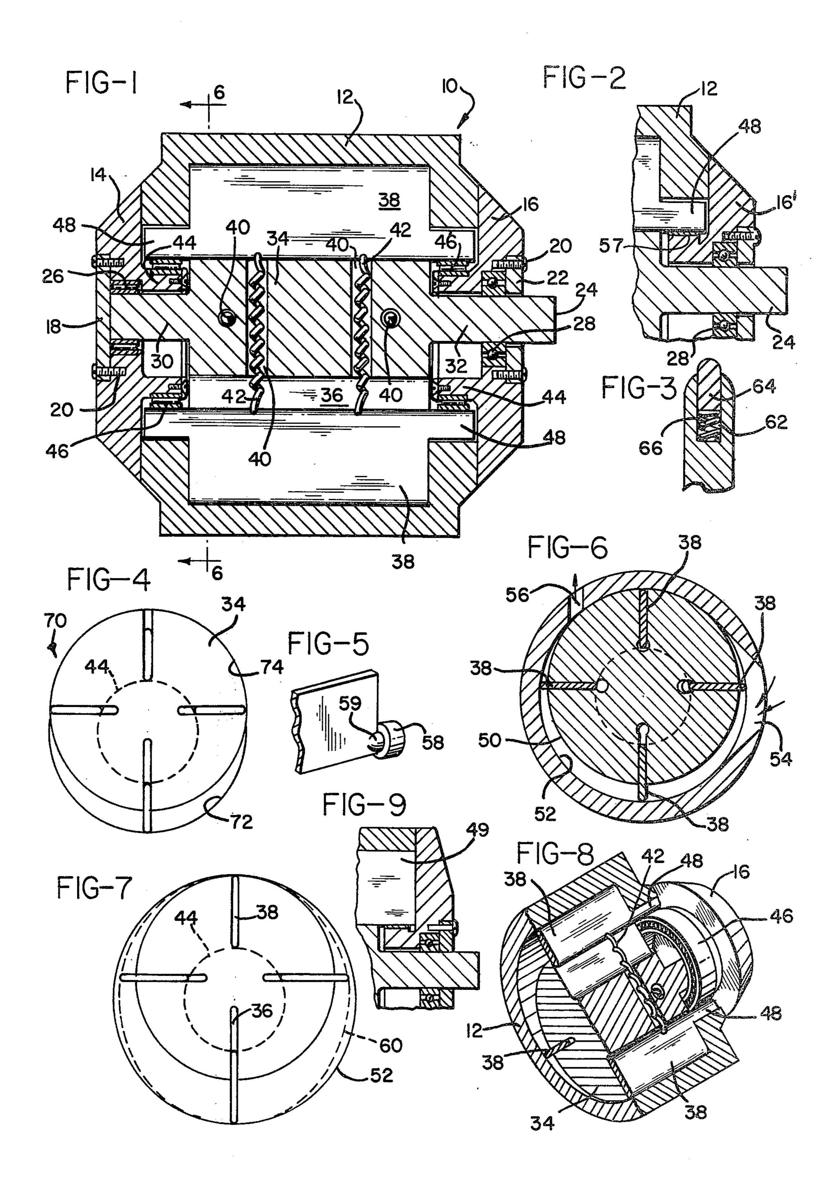
ROTARY CAM-ACTUATED VANE MACHINE
