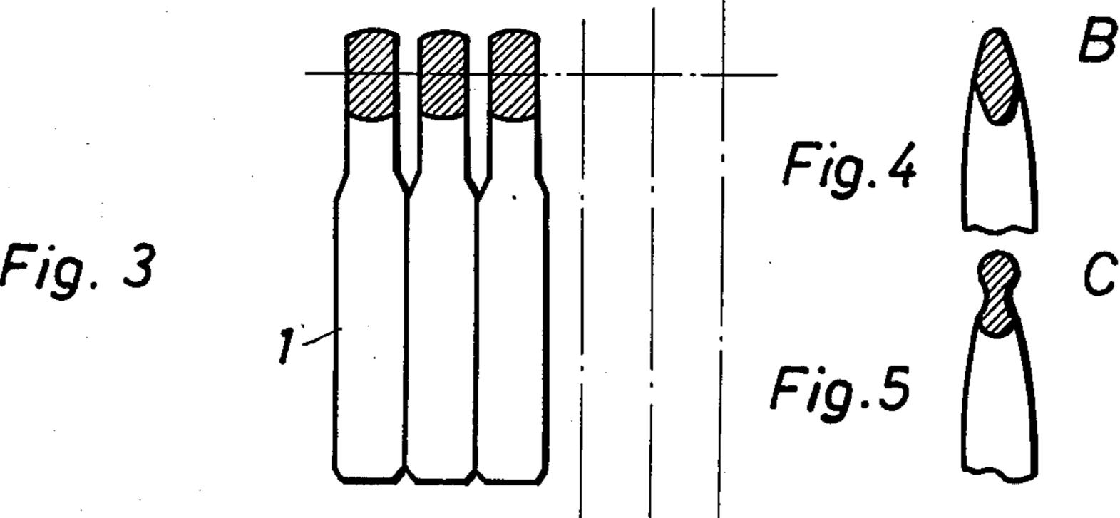
This invention relates to a U-shaped clip which is intended to close bags, flexible tubes or the like and has 5 been made from a piece of wire which is constant in
