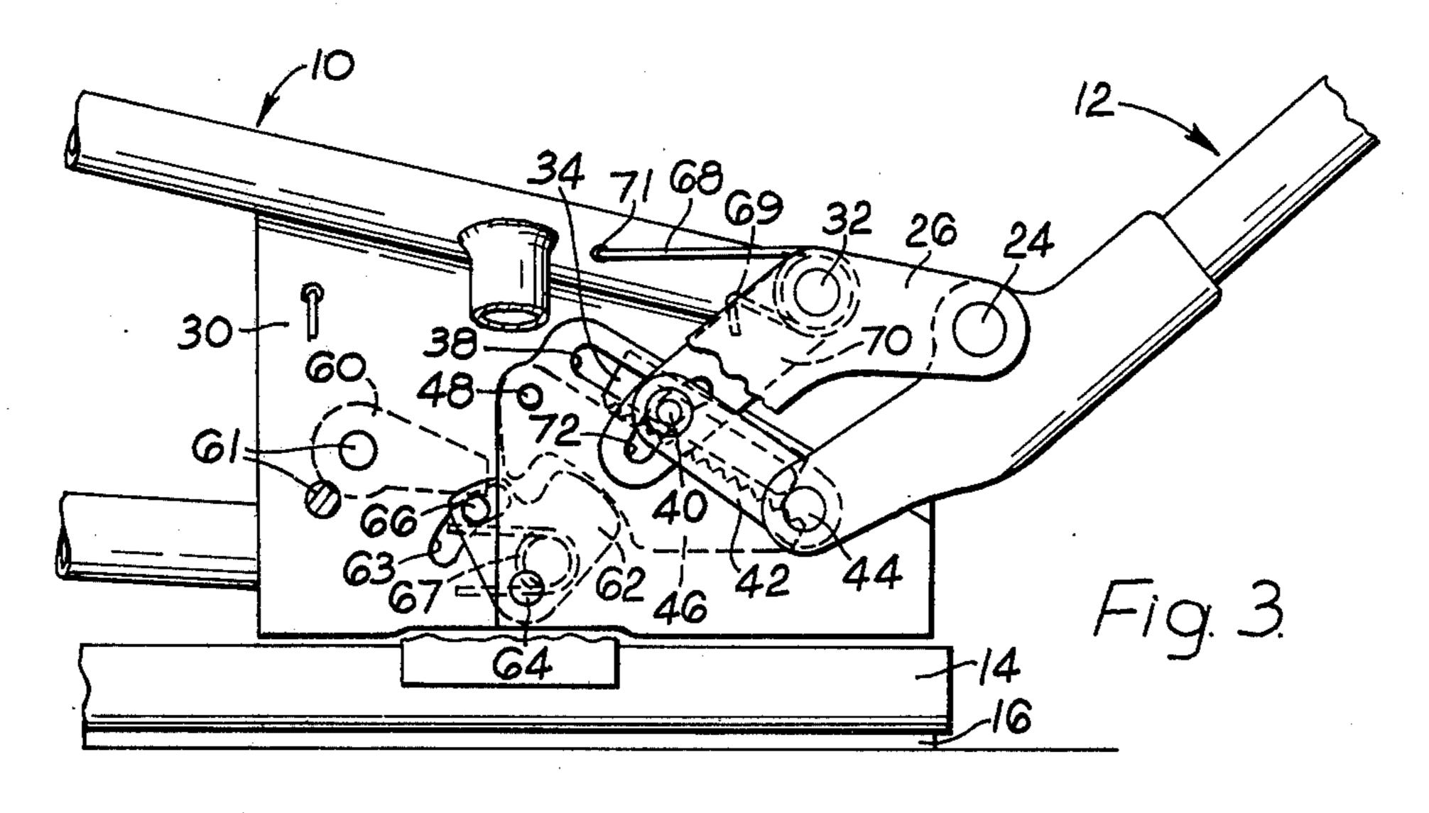
This invention relates to vehicle seats and, in particular, to mechanisms for incorporation in such seats so as 5 to enable the backrest to be adjusted in inclination relative to the seat base and/or to be folded with accompa-
